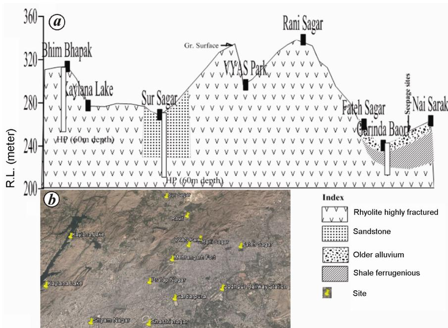
**Figure 2.** *a*, Reduced level of seepage locations and Kaylana lake along with geological setting; *b*, Sites along with Kaylana lake.
