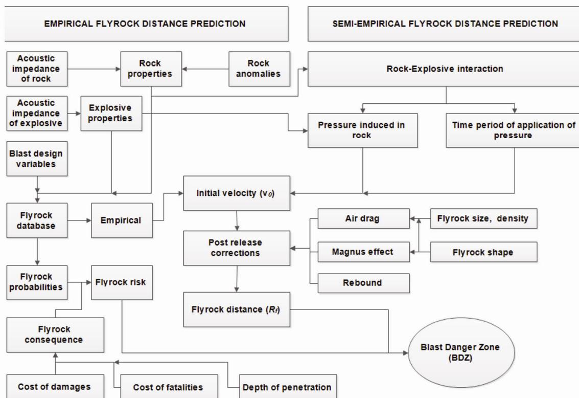
**Figure 2.** Flyrock and Blast Danger Zone prediction mechanism.
