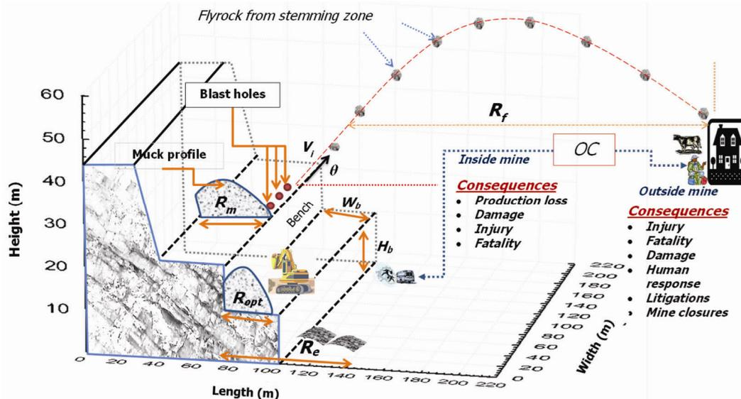
**Figure 1.** Description of throw, excessive throw and flyrock.  $H_b$ , Bench height;  $W_b$ , Bench width;  $R_e$ , Excess throw;  $R_f$ , Flyrock distance;  $R_{opt}$ , Optimum throw for loading efficiency;  $V_c$ , Exit or maximum velocity of flyrock;  $\theta$ , Launch angle of flyrock and OC, Objects of concern.
