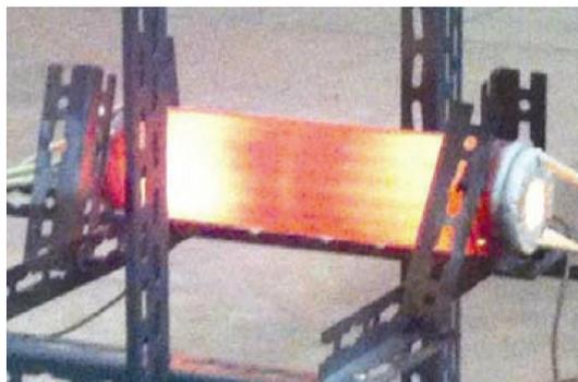
**Figure 2.** Visible image of an E-CAT HT during November 2012 prior to its self-destruction by internal melting.
