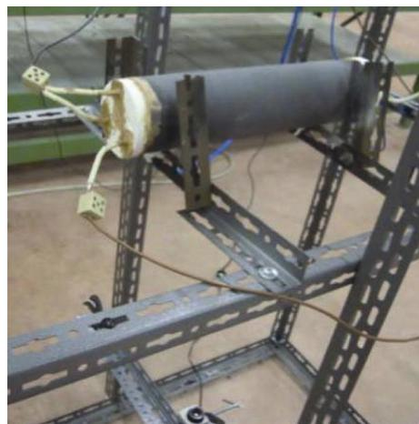
**Figure 3.** Visible image of E-CAT HT with the white electrical leads on the left and the IR camera on the floor.
