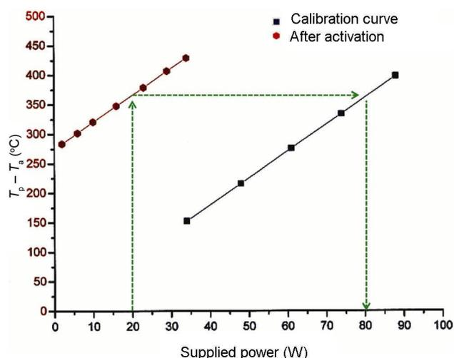
**Figure 1.** Temperature ( $T_p$ ) in the core of the experiment relative to ambient temperature ( $T_a$ ) for two cases, a calibration curve and a Ni rod that had been activated. Only 20 W of input power is needed for the activated rod to attain the same temperature as produced by 80 W of power input for the calibration run. This indicates an excess power of 60 W for the 20 W of input electrical power.
