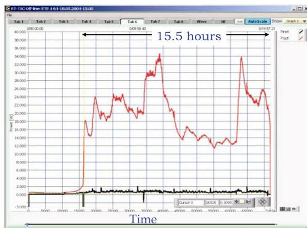
**Figure 2.** Plots of power in (black) and out (red) for an experiment that gave an energy gain of 26. The vertical scale is in W up to 40 W (2 W/division).
