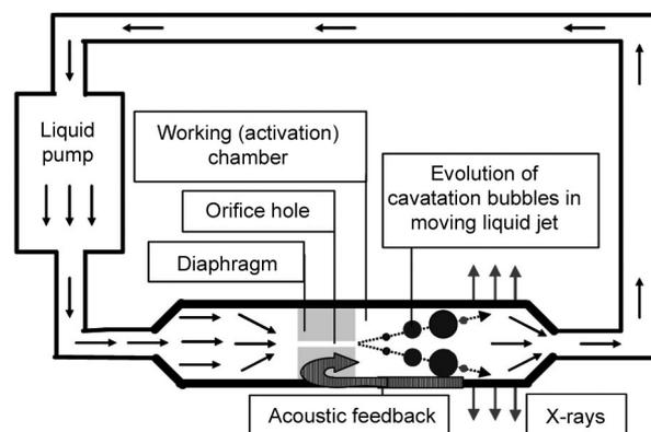
**Figure 1.** Experimental set-up for the study of radiative phenomena at cavitation in moving spindle oil.
