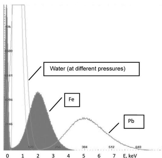
**Figure 3.** Spectra of X-radiation from different surfaces at cavitation of fast water jet at 600 atm.
