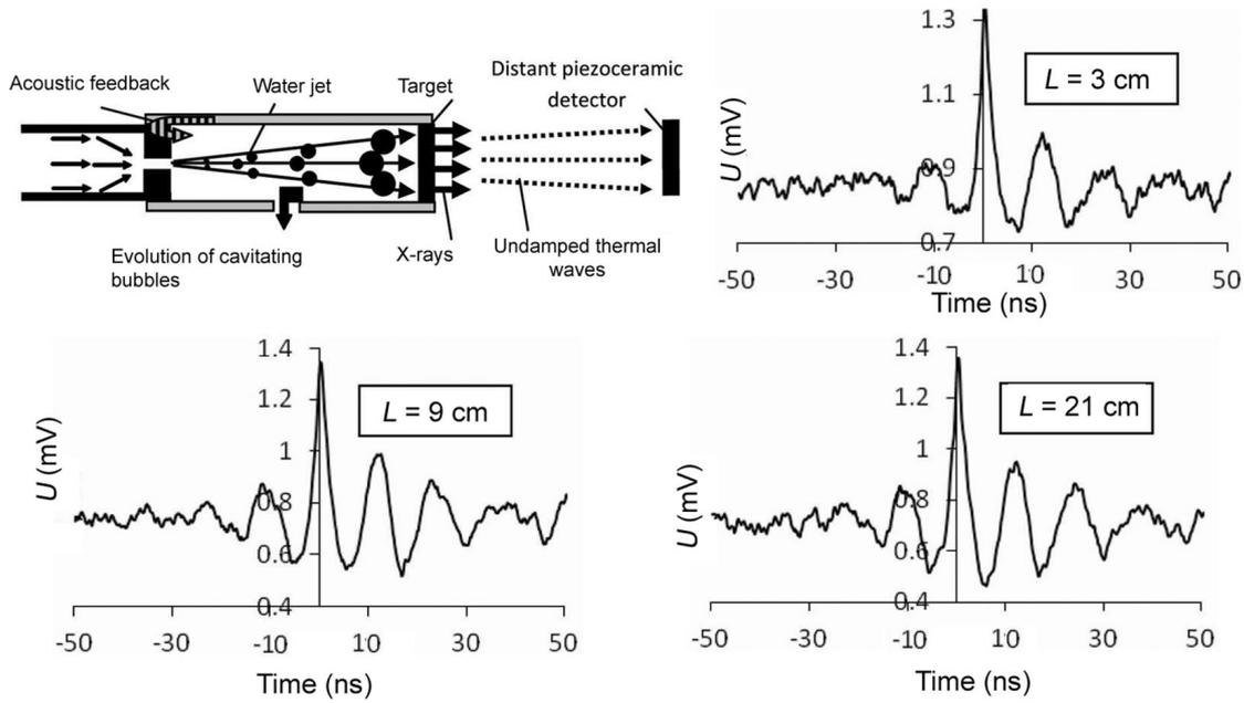
**Figure 6.** Experimental set-up for study of X-rays and undamped thermal waves at cavitation of fast water jet and high-frequency signals registered in air at different distances  $L$ .
