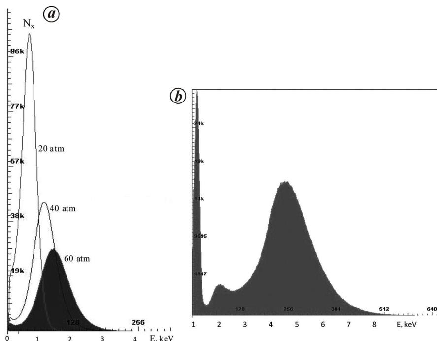
**Figure 2.** X-ray spectrum detected outside the cavitation chamber: *a*, At different oil pressures; *b*, At  $P = 37$  atm in the presence of copper powder on the outer surface of the chamber.  $N_x$  is the total number of X-ray quanta detected for 5 min.
