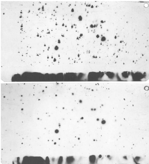
**Figure 5.** Images on plane X-ray (two films stacked tightly in a light protective paper envelope and mounted behind the steel screen). The appear film is closer to the screen.
