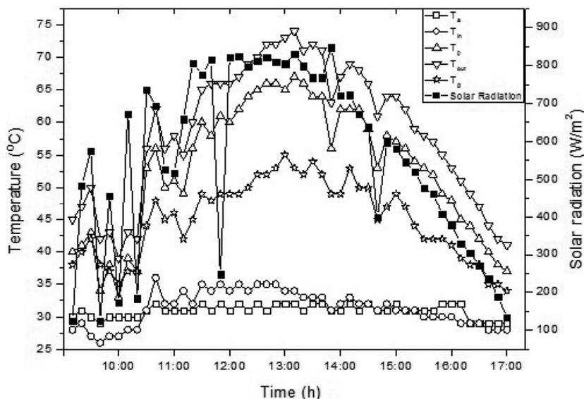
Figure 5. Temperature and solar radiation versus time (with load).
