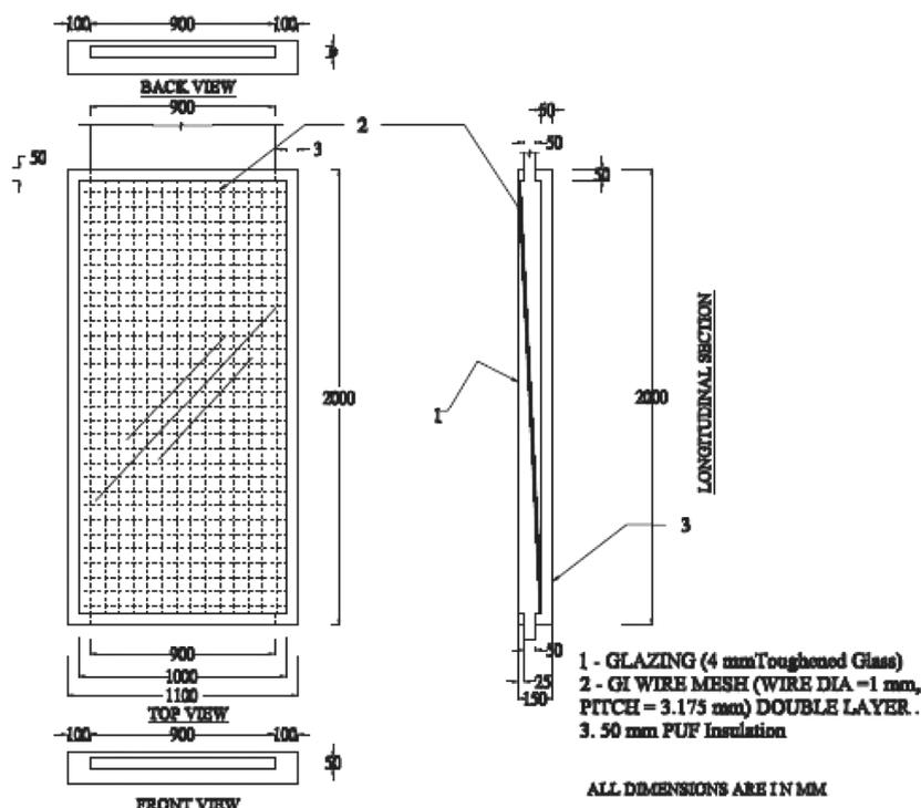
Figure 1. Schematic diagram of the wire mesh solar air heater.
