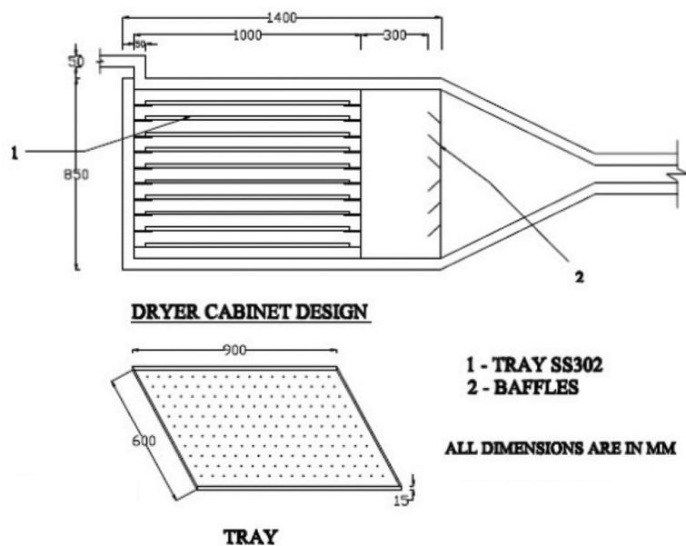
**Figure 3.** Schematic diagram of the drying cabinet and tray.
