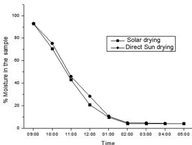
Figure 6. Drying curve for the sample.
