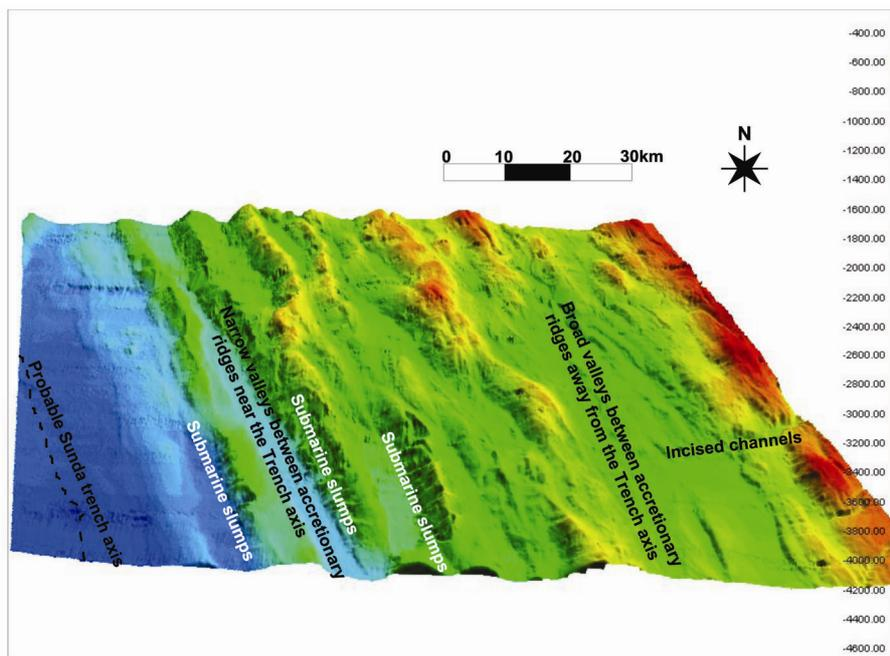
**Figure 1.** Morphometric set up of the Andaman accretionary prism (AAP) showing the different tectonic elements. Fluid migration along the decollments are also shown.
