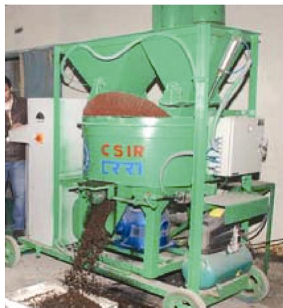
**Figure 3.** Portable pothole repair machine.
