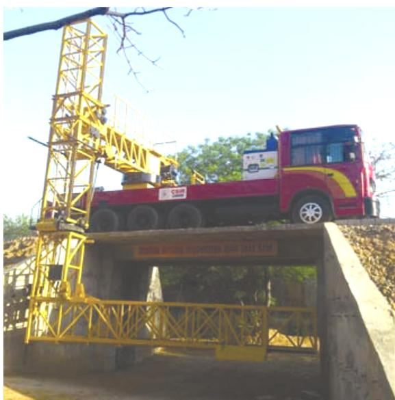
**Figure 2.** Mobile bridge inspection unit.
