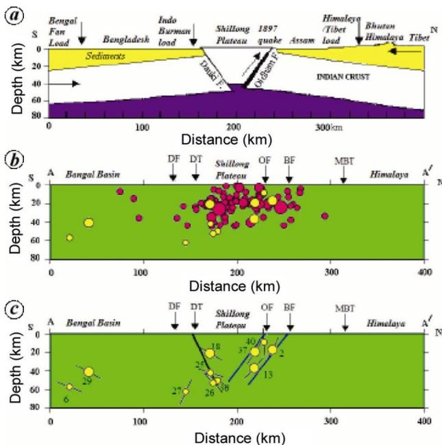
**Figure 11.** a, Pop-up tectonic model of the Shillong plateau<sup>37</sup>. b, Earthquakes beneath the Shillong plateau. c, Fault planes of the annotated earthquakes indicate that DT and BF are the boundary faults<sup>44</sup>.
