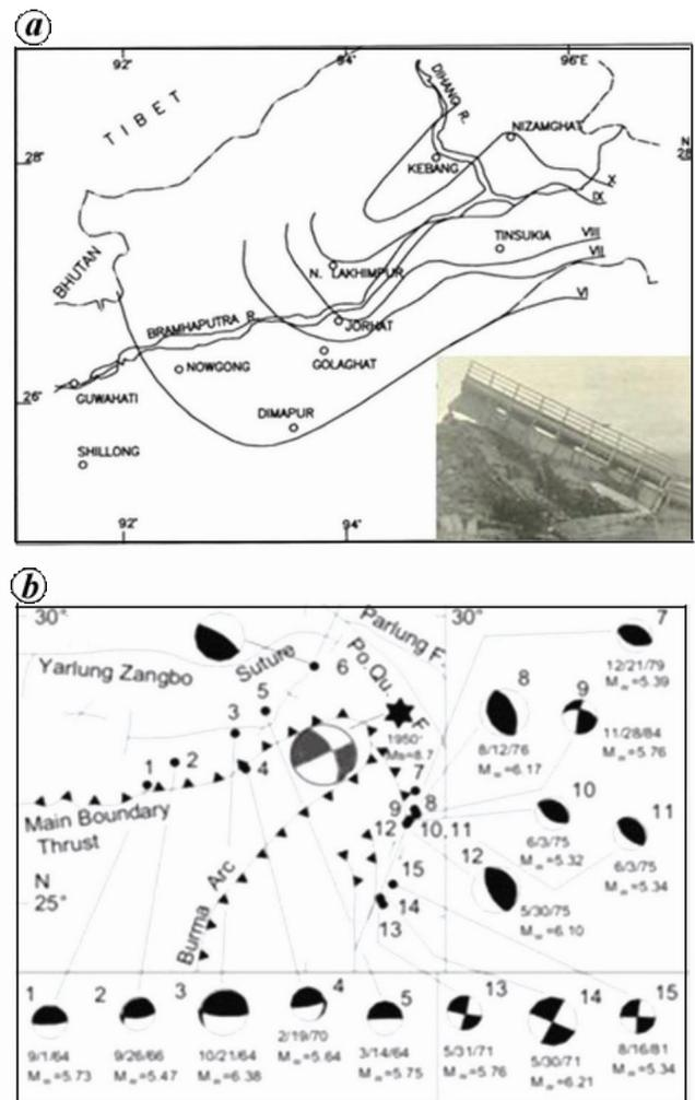
**Figure 12.** a, Isoseismal map of the 1950 Assam earthquake. (Inset) Damaged bridge in the maximum intensity zone. b, Fault plane solutions of the earthquakes in the eastern syntaxis zone (compiled by Kayal<sup>24</sup>).
