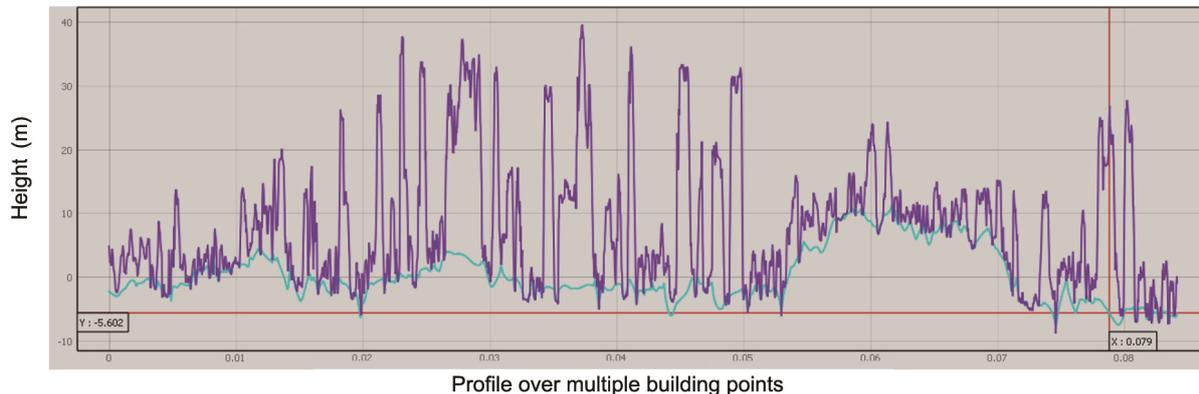
Figure 4. DEM and DTM profile over wider building coverage.
