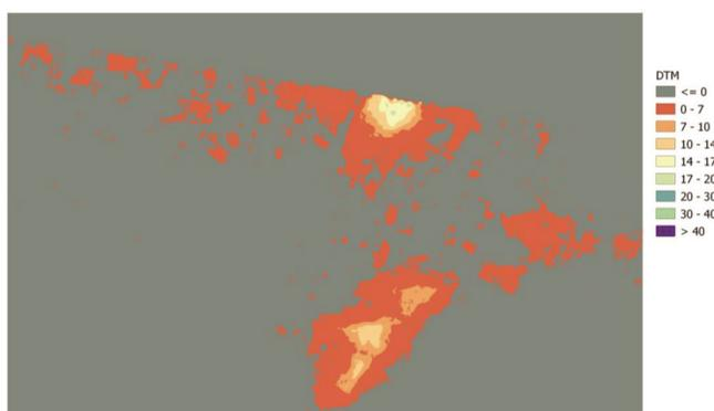
**Figure 2.** Digital terrain model (DTM) height (m) results after slope filtering.
