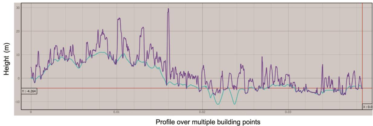
**Figure 3.** DEM and DTM profile over selected buildings.
