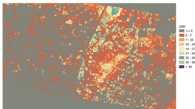
**Figure 1.** Digital elevation model (DEM) results and building height (m) classification using DEM data.
