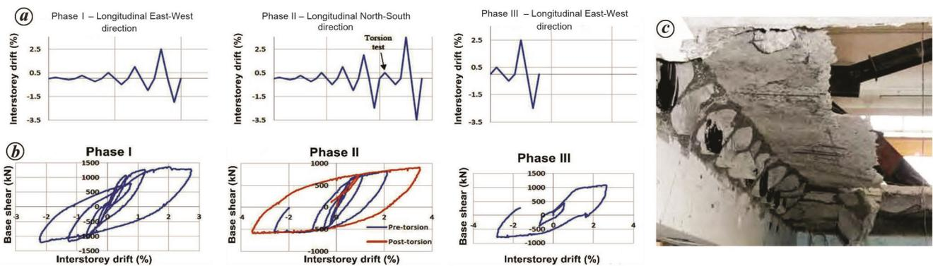
Figure 6. Performance of the super-assembly test<sup>45</sup>: a, Loading protocol; b, Hysteresis loop; c, Failure mode showing starters and end of the HC units remain attached to the east beam.
