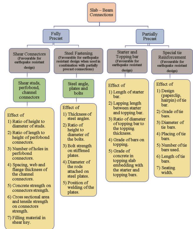
**Figure 1.** Quantitative design parameters influencing the performance of slab to beam connection.
