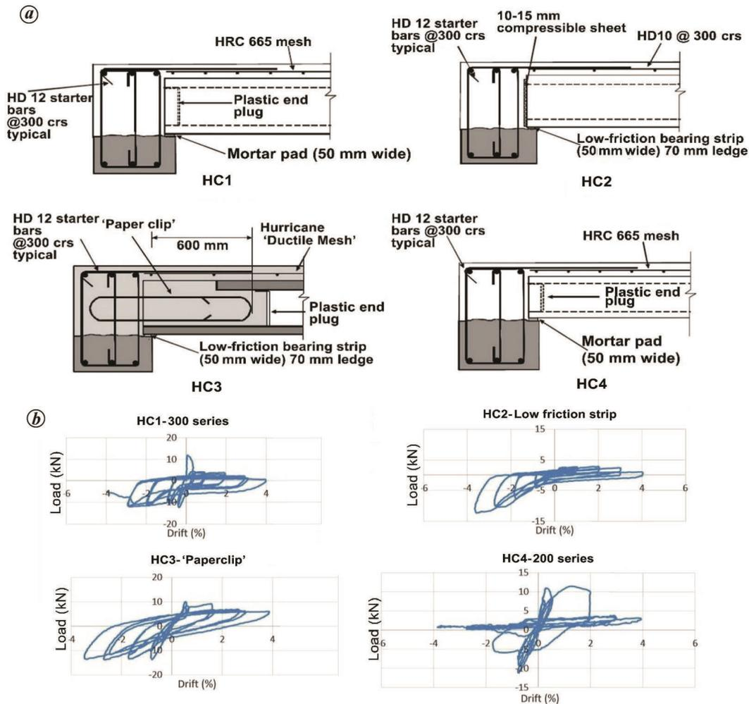
Figure 7. Details of sub-assembly<sup>46</sup>: *a*, Connection details; *b*, Hysteresis performance of the tested connection.
