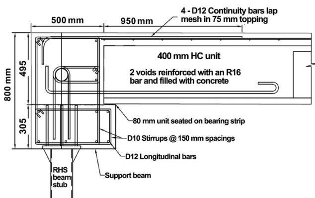
Figure 9. Recommended connection detail for 400 HC from NZS 3101:2006 (ref. 13).
