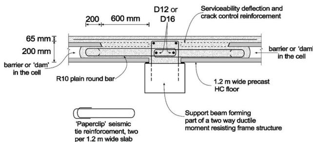
Figure 4. 'Paperclip' tie connection detail<sup>42</sup>.
