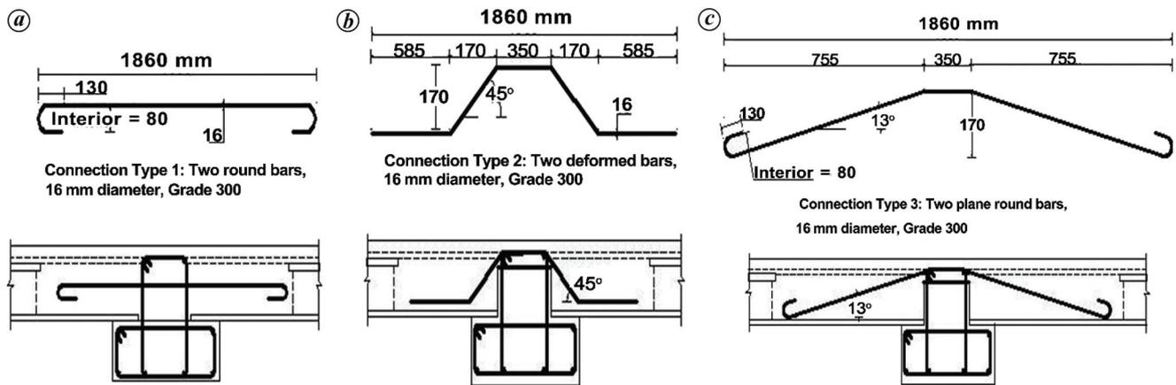
Figure 3. Special tie connection details of test specimen<sup>40</sup>: a, Type 1, Hanger tie; b, Type 2, Saddle tie with 45° bend; c, Type 3, Saddle tie with 13° bend.
