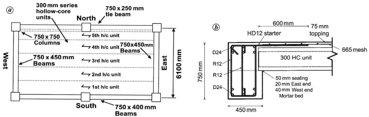
Figure 5. Details of super-assembly<sup>45</sup>: a, Plan; b, Connection detail.
