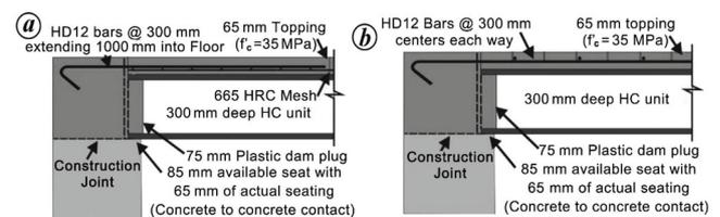
**Figure 2.** Connection details of test specimen<sup>38</sup>: a, HCW1; b, HCW2.
