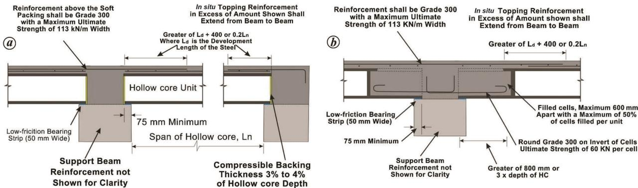
Figure 8. ‘Acceptable solution’<sup>51</sup> proposed by New Zealand concrete standards: a, First solution; b, Second solution.
