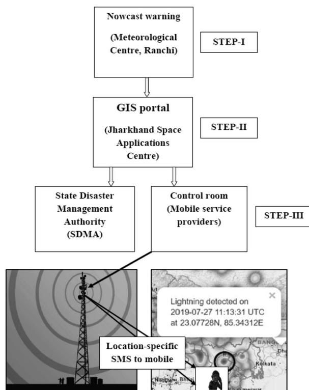
Figure 5. Flow diagram of location-specific nowcast and SMS-based dissemination system (LN-SMS-DS).
