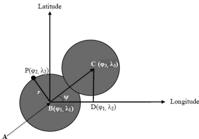
Figure 7. Schematic diagram of extrapolation of thunderstorm cell.
