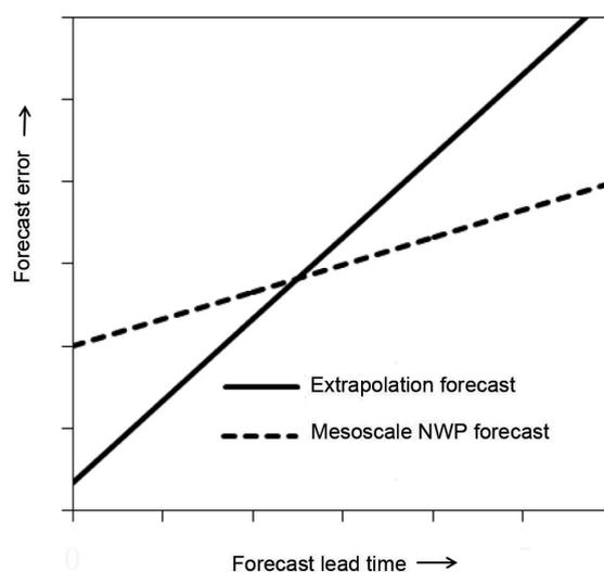
Figure 4. Schematic representation of the characteristics of error distribution of extrapolation forecast and mesoscale NWP forecast.
