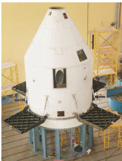
**Figure 13.** Crew Module Fairing with composite grid fins in deployed condition.
