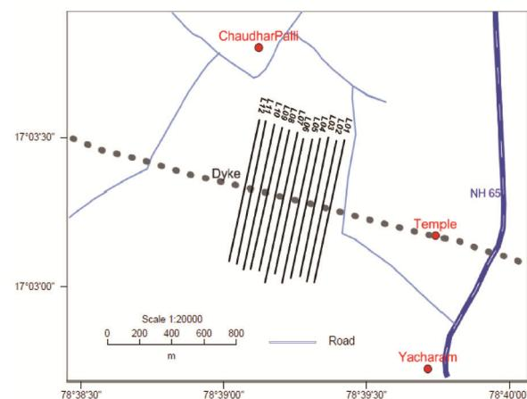
**Figure 2.** Study area showing magnetic profile (solid black lines) orthogonal to the dyke (black dotted line).
