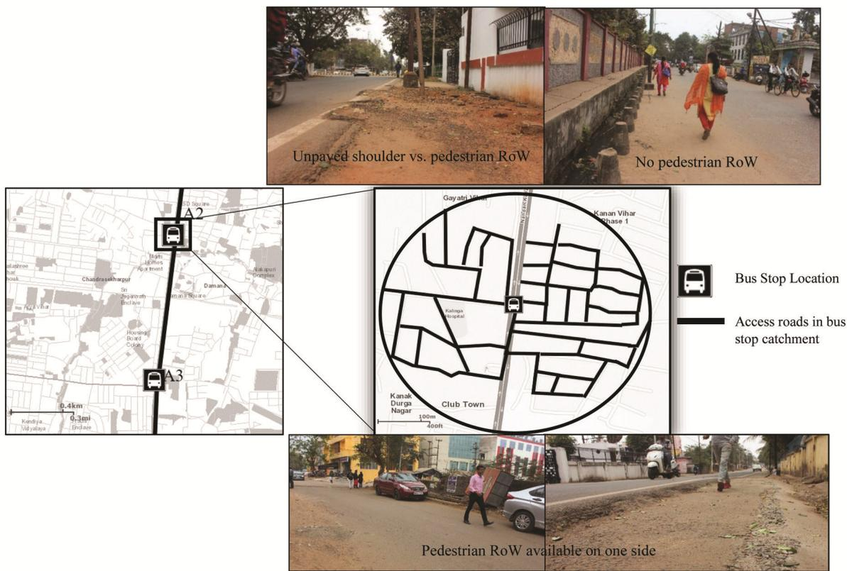
**Figure 2.** Access roads showing geometric features of varying nature in a bus stop catchment located at Chandrashekharpur area, Bhubaneswar (A2 in Figure 1).
