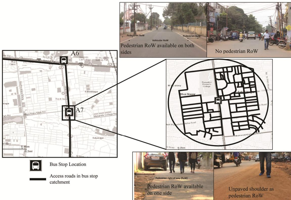
**Figure 3.** Access roads showing geometric features of varying nature in a bus-stop catchment located at Saheed Nagar, Bhubaneswar (A7 of Figure 1).
