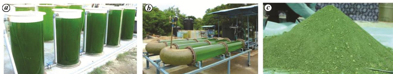
**Figure 1.** Marine *Chlorella vulgaris* (NIOT-74) cultured in: *a*, continuous flow bubble column photobioreactor; *b*, tubular photobioreactor; *c*, harvested biomass under outdoor conditions.
