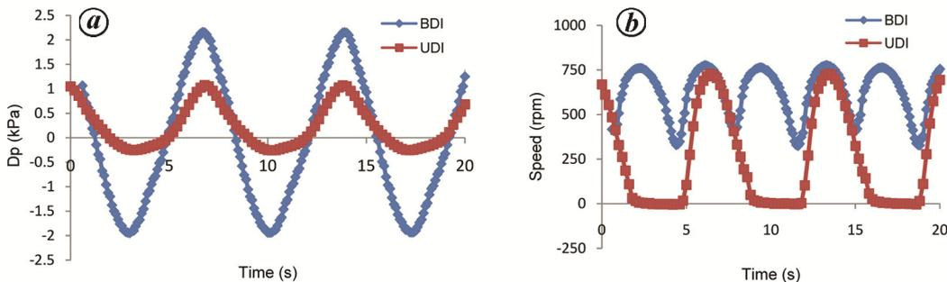
Figure 4. a, Time series of Dp across the turbine; b, Time series of speed across the turbine.
