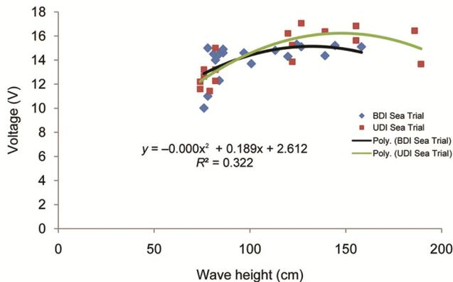
**Figure 10.** Generated voltage for different wave heights.
