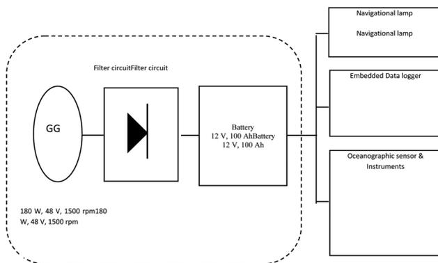
Figure 1. Schematic of power take off system.
