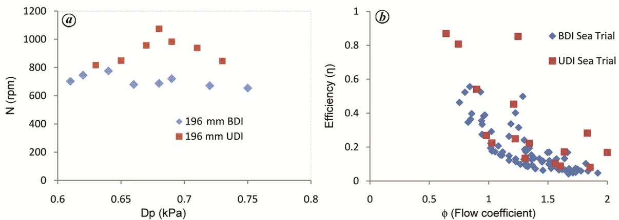
**Figure 9.** *a*, Turbine speed versus  $D_p$ . *b*, Turbine efficiency versus flow coefficient.
