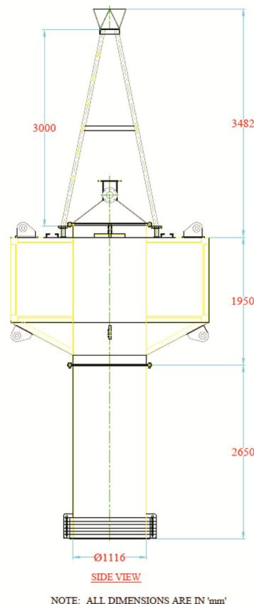
Figure 7. Line diagram of navigational buoy.
