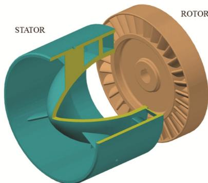
Figure 2. CAD image of the wave energy turbine.
