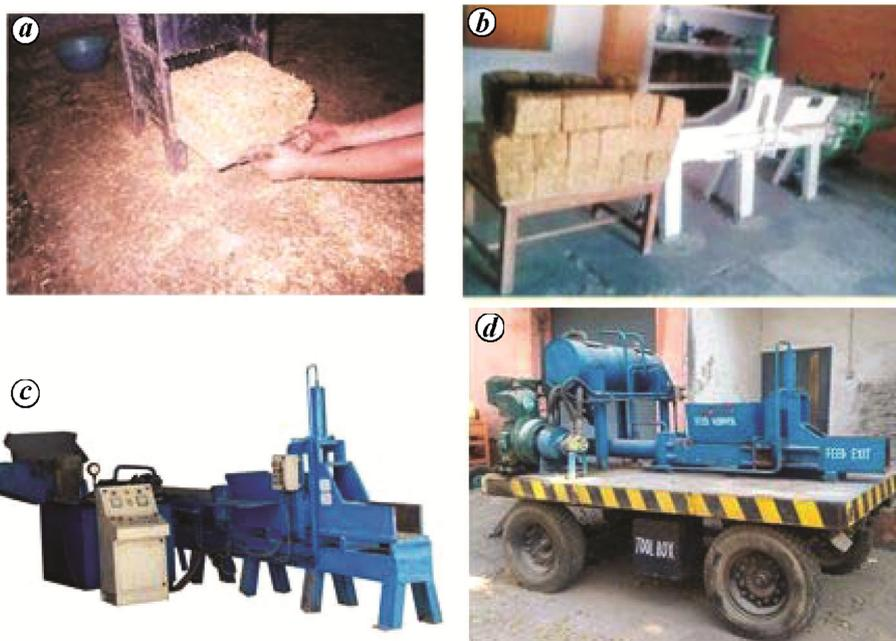
**Figure 2.** *a*, Manually operated feed block-making machine (source: Khan *et al.*<sup>14</sup>). *b*, Power-operated feed block-making machine (Source: Bohra *et al.*<sup>24</sup>). *c*, Electrically powered hydraulic plunger/piston press-type feed block-making machine (source: Bohra *et al.*<sup>24</sup>). *d*, IC engine-operated, tractor trolley-mounted hydraulic plunger/piston press-type feed block-making machine.
