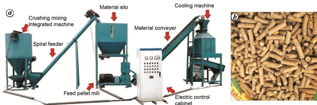
**Figure 4.** a, Pictorial view of industrial CF pellet production (source: Anon.<sup>25</sup>). b, The 8 mm diameter cattle feed pellets.
