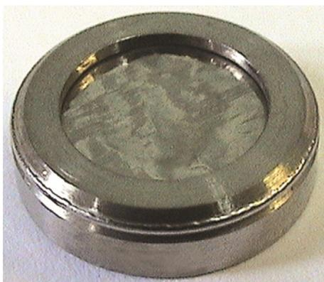
**Figure 5.** Encapsulated  $^{244}\text{Cm}$  alpha source.
