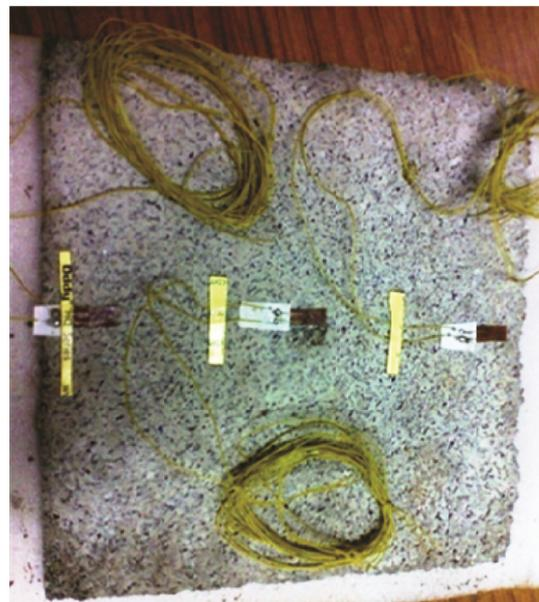
Figure 1. Model raft along with the strain gauges.
