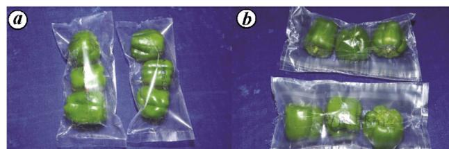
Figure 2. a, PLA + PEG MA package. b, PLA + PBAT (10%) MA package.
