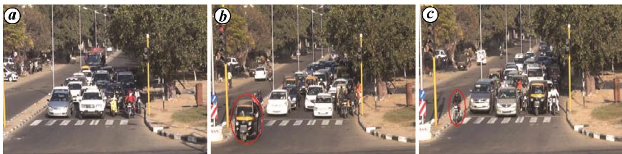
Figure 3. Vehicle stoppage position (a) before and (b, c) after the approach stop line during red interval.
