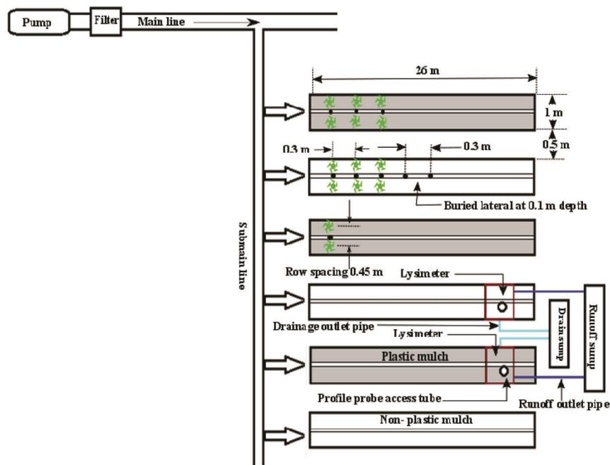
Figure 1. Subsurface drip irrigation layout with lysimetric set-up.
