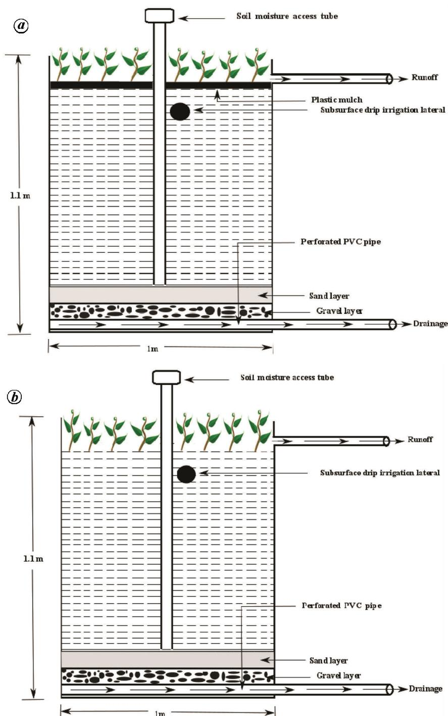
**Figure 2.** Drainage lysimeter under (a) plastic mulch and (b) non-plastic mulch conditions.
