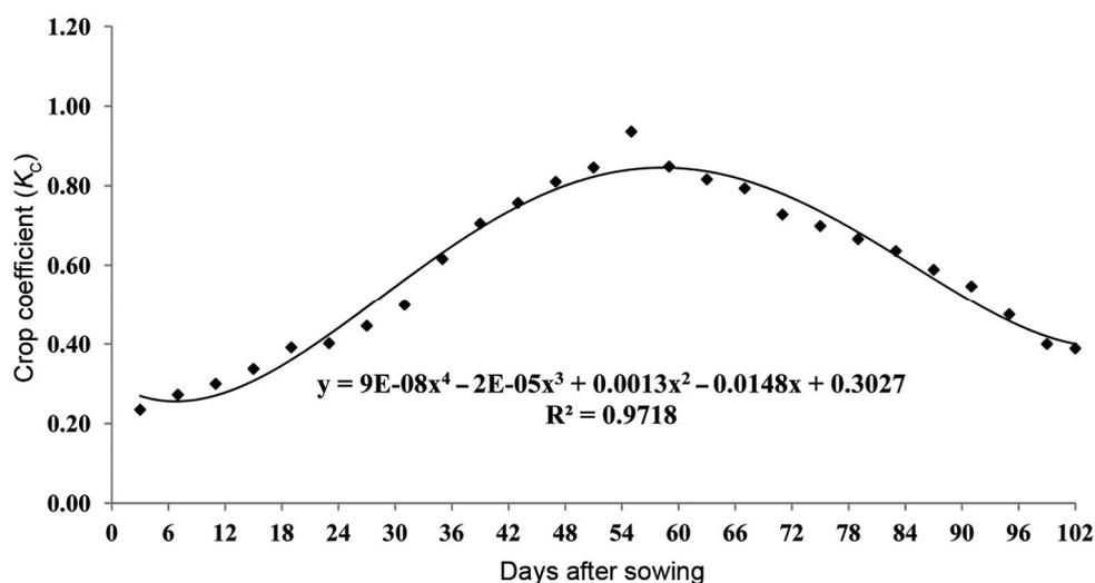
**Figure 7.** Average crop coefficient ( $K_C$ ) versus days after sowing regression curve for 2016 and 2017 seasons under plastic mulch condition.
