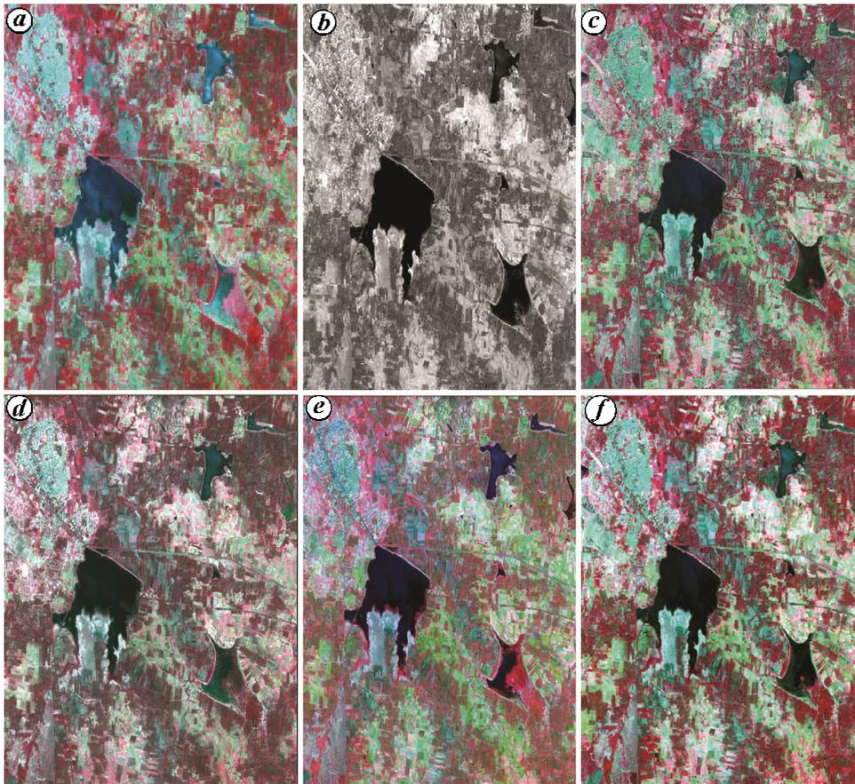
**Figure 1.** The fusion results of a satellite image. *a*, Multispectral image; *b*, Panchromatic image. *c*, Wavelet method; *d*, Principal component analysis; *e*, Spatial correlation analysis; *f*, RWPCA-WT method.
