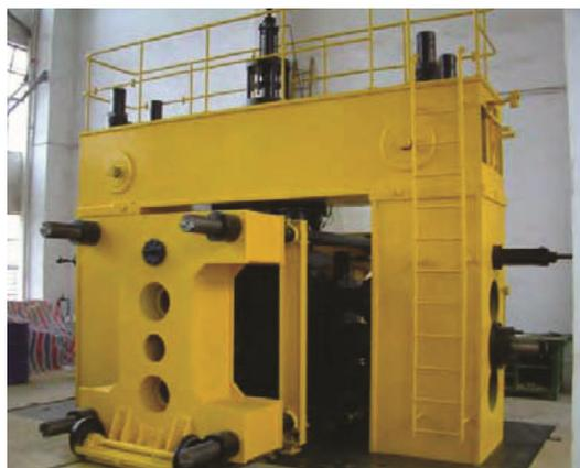
Figure 2. Large scale true triaxial servo loading system.
