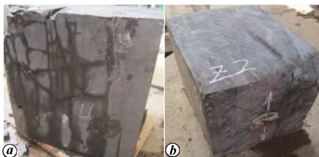
**Figure 10.** Fracture geometry of hydraulic fracturing of shale specimens.
