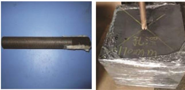
**Figure 8.** Symmetrical slotted steel pipe and the simulation casing.
