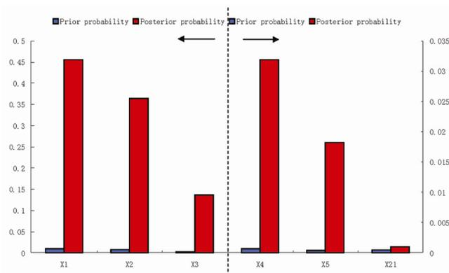
Figure 8. The probability changes of critical basic events of rail haulage accidents.
