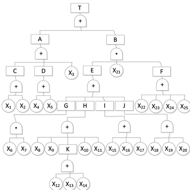
**Figure 6.** The fault tree of a rail haulage accident.
