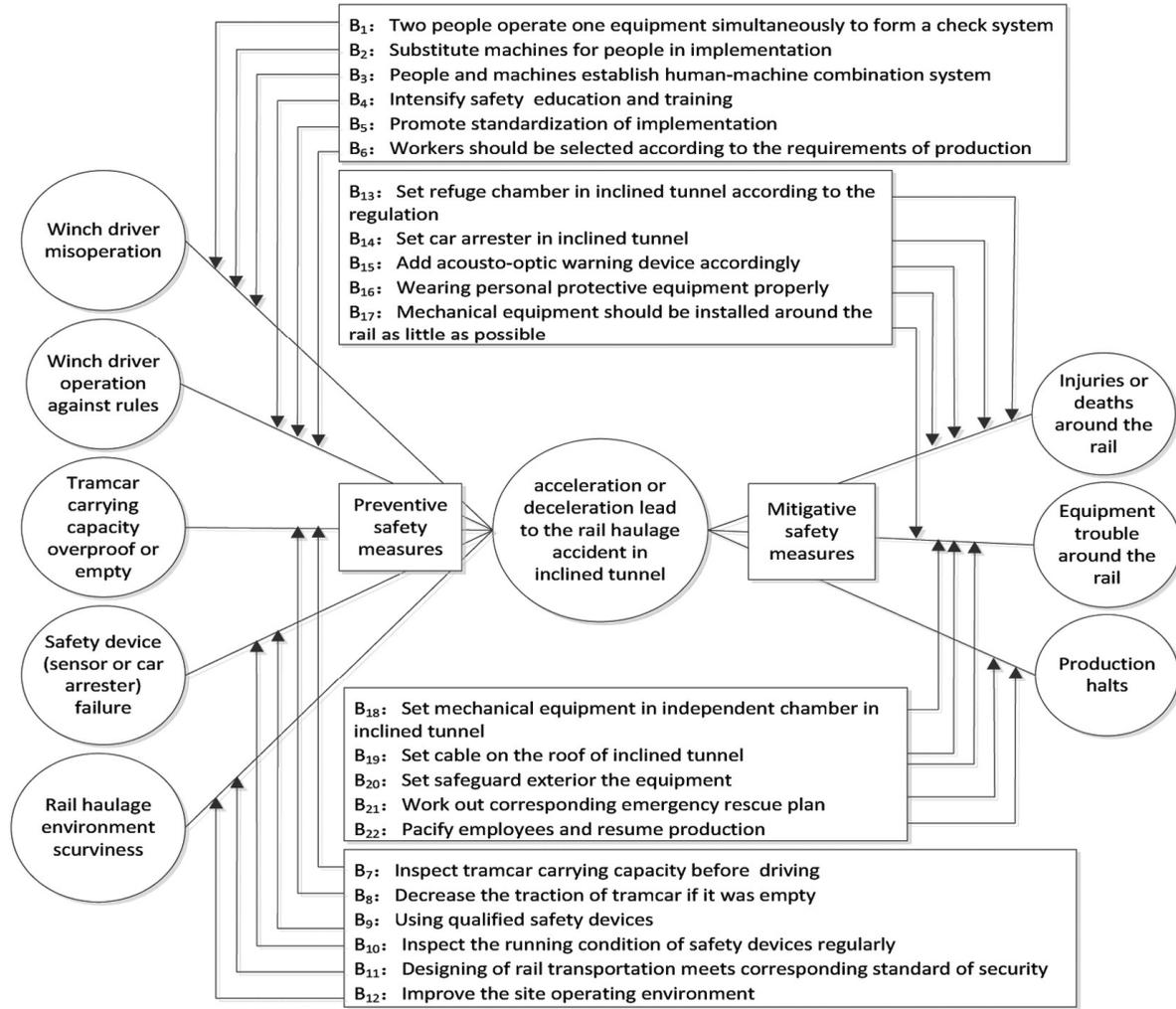
Figure 9. Bow-tie analysis of acceleration or deceleration.
