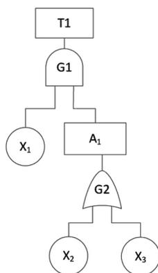
Figure 1. A simple fault tree.
