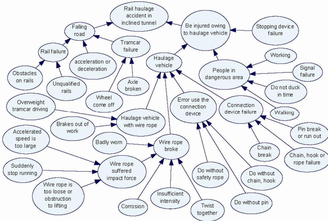
Figure 7. Bayesian network of the rail haulage accident in an inclined tunnel.
