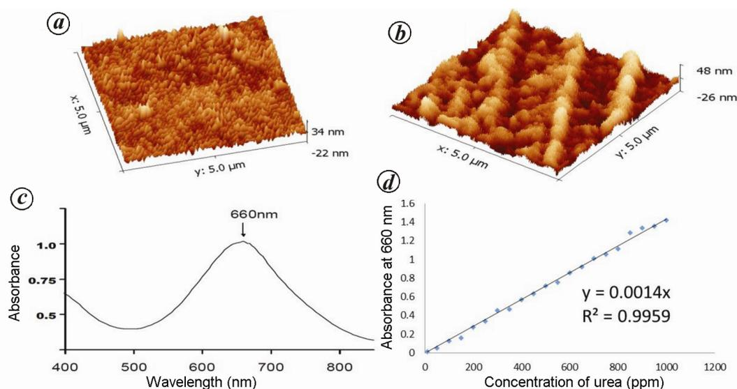
**Figure 2.** AFM images of nanocellulose reinforced starch/polyvinyl alcohol film before (a) and after (b) urease immobilization. The spectrum (c) shows the response of biosensor to urea with lambda max at 660 nm and (d) shows the linearity curve of biosensor.
