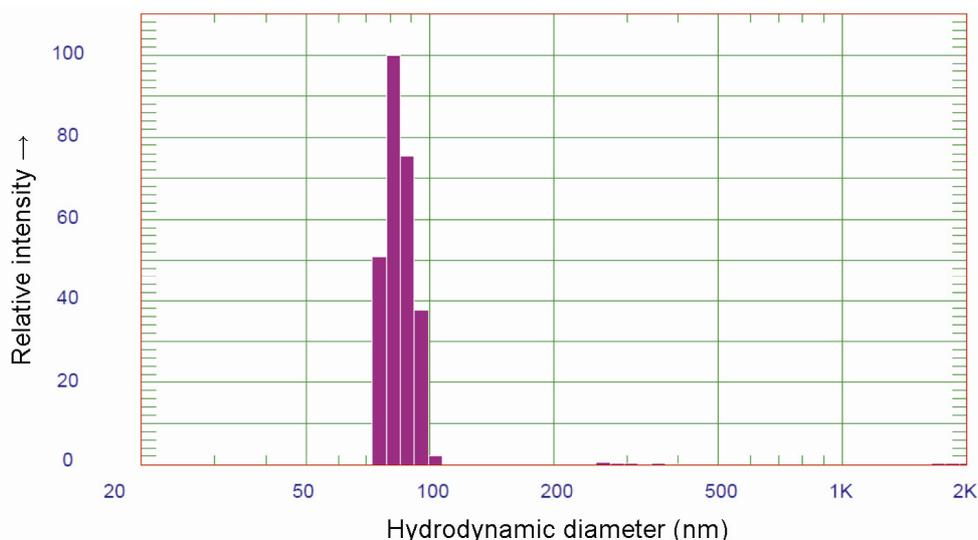
**Figure 1.** Particle size distribution of nanocellulose analysed by DLS particle size analyser.
