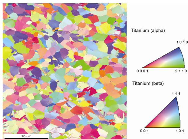
**Figure 3.** Electron back scattered diffraction image showing uniform fine  $\alpha + \beta$  microstructure with random texture in Ti6Al4V.
