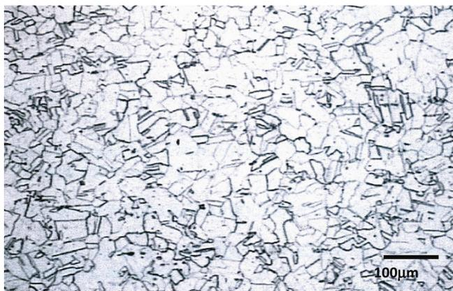
**Figure 6.** Microstructure showing fine austenitic grain matrix in sample representative of large-sized Inconel-718 forgings.
