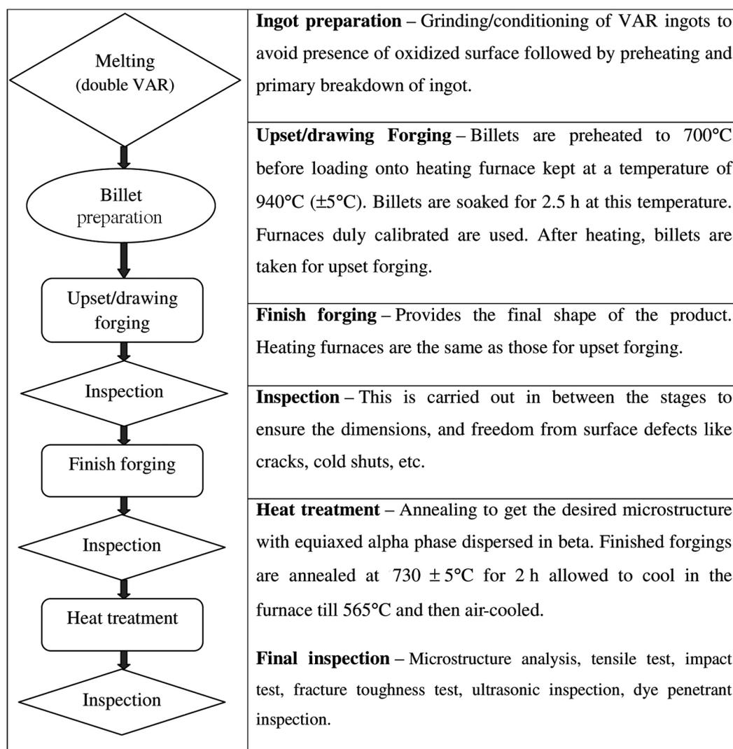
**Figure 1.** Process flow chart for realization of Ti6Al4V forgings.
