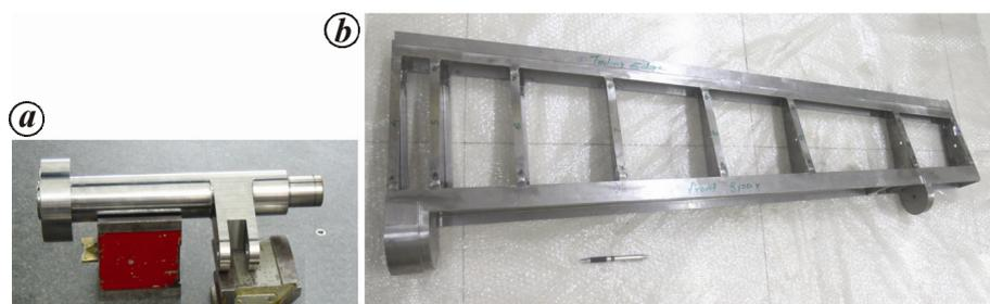
Figure 4. (a) Elevon shaft and (b) Elevon torsion box used in RLV-TD.
