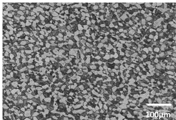
**Figure 2.** Microstructure of Ti6Al4V shows primary  $\alpha$  phase in transformed  $\beta$  matrix.
