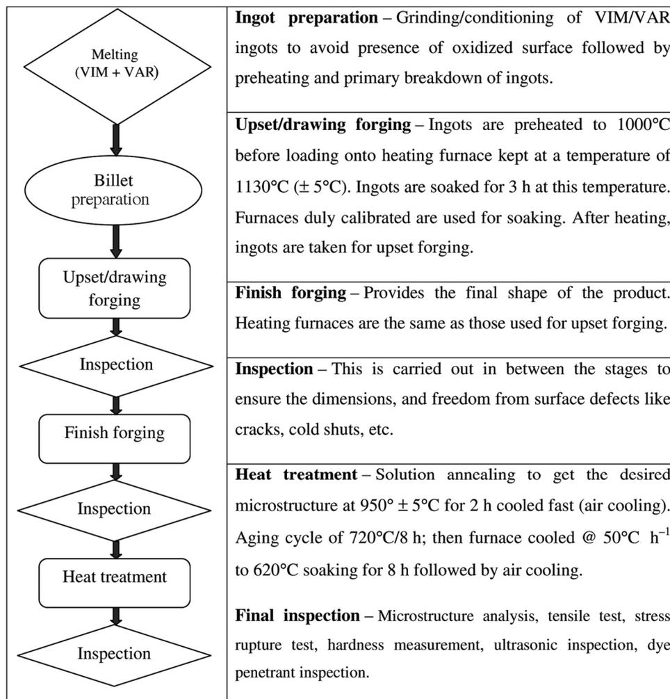
Figure 5. Process flow chart for realization of Inconel-718 forgings.
