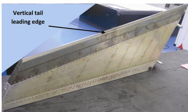
**Figure 7.** A vertical tail leading edge fabricated from Inconel-718 forged block of size  $60 \times 120 \times 1420 \text{ mm}^3$  used in RLV-TD.
