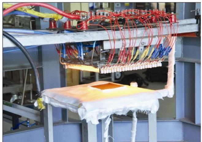
**Figure 5.** Testing radio frequency performance at high temperature.
