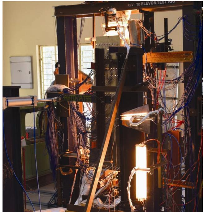
**Figure 3.** Elevon thermo-structural test.
