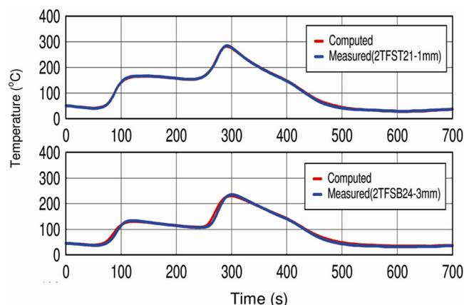
Figure 9. Comparison of computed and measured temperature histories on silica tile.
