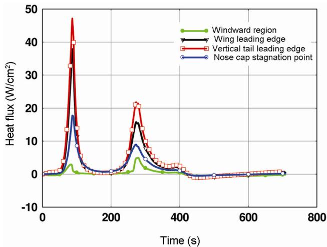
**Figure 2.** Cold wall heat flux estimated at various locations of RLV-TD.
