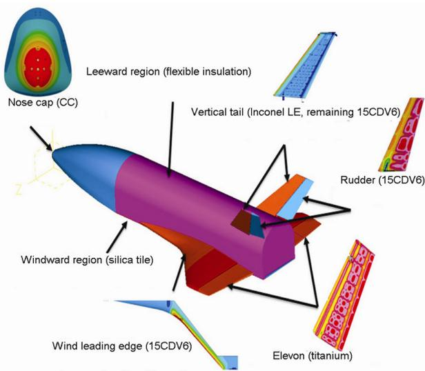
**Figure 1.** Various structures of RLV-TD.
