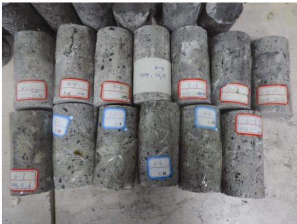
**Figure 4.** Failure morphology of samples.
