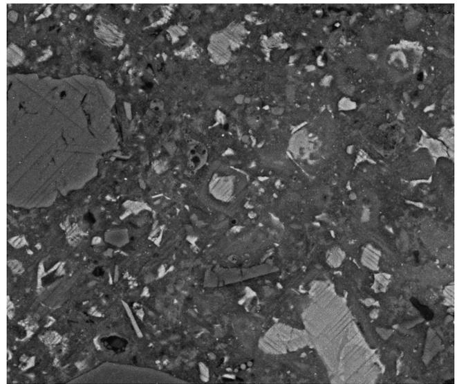
**Figure 16.** BSE image of C1HC after 28 days of hydration (width of field  $\approx 275 \mu\text{m}$ ).
