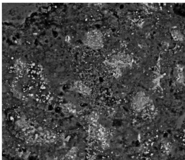
**Figure 19.** BSE image of C1AC after 1 day of hydration (width of field  $\approx 275 \mu\text{m}$ ).
