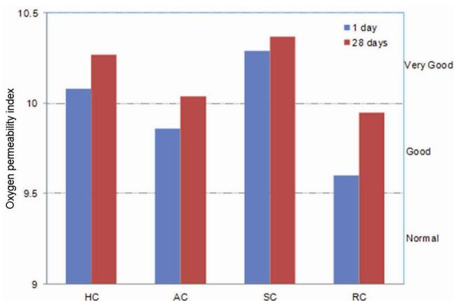
**Figure 9.** Oxygen permeability index results of HESC with cement C1.
