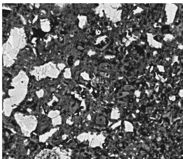
**Figure 13.** BSE image of C1RC after 1 day of hydration showing high porosity and unhydrated cement grains (width of field  $\approx$  275  $\mu$ m).
