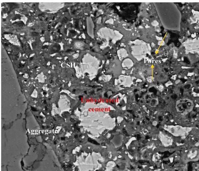
**Figure 14.** BSE image of C1RC after 28 days of hydration (width of field  $\approx 275 \mu\text{m}$ ).
