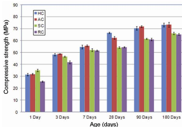
**Figure 1.** Compressive strength results of HESC mixtures with cement C1.
