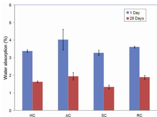
**Figure 12.** Water absorption of concretes with cement C2 on days 1 and 28.
