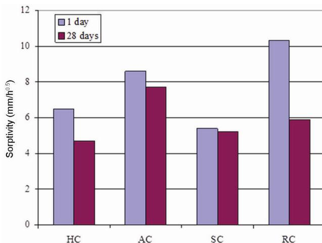
**Figure 4.** Sorptivity values of concretes containing cement C2 on days 1 and 28.
