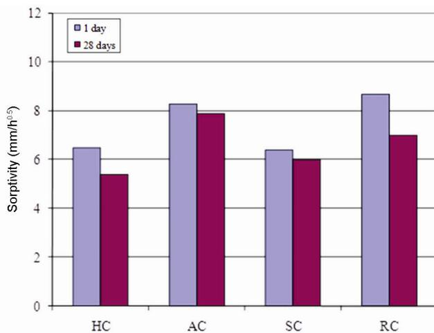
**Figure 3.** Sorptivity values of concretes containing cement C1 on days 1 and 28.
