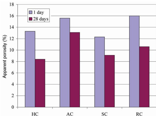
**Figure 6.** Apparent porosity of HESC containing cement C2 on days 1 and 28.
