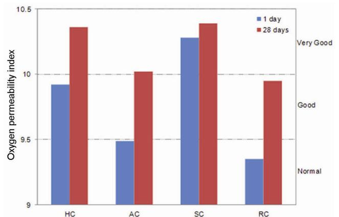
**Figure 10.** Oxygen permeability index results of HESC with cement C2.
