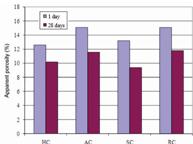
**Figure 5.** Apparent porosity of HESC containing cement C1 on days 1 and 28.
