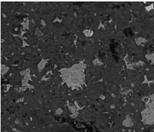
**Figure 15.** BSE image of C1HC after 1 day of hydration (width of field  $\approx 275 \mu\text{m}$ ).
