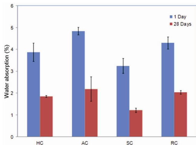
**Figure 11.** Water absorption of concretes with cement C1 on days 1 and 28.
