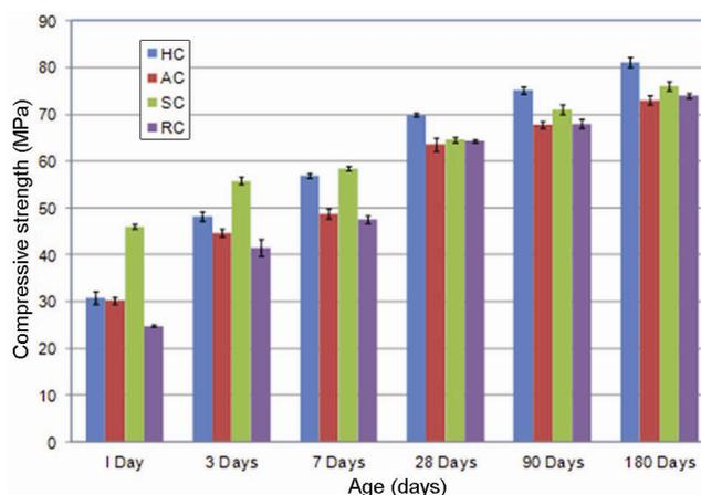
**Figure 2.** Compressive strength results of HESC mixtures with cement C2.
