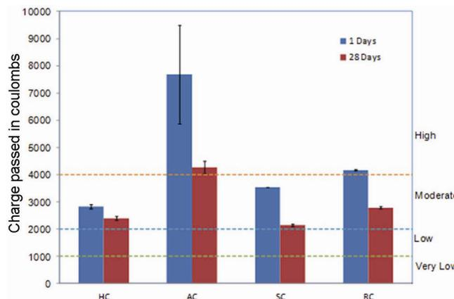
**Figure 8.** Chloride permeability values of concretes with cement C2.
