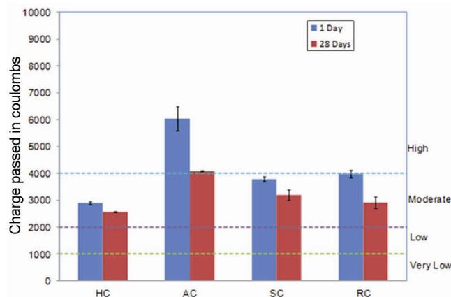
**Figure 7.** Chloride permeability values of concretes with cement C1.
