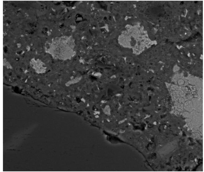
**Figure 17.** BSE image of C1SC after 1 day of hydration (width of field  $\approx 275 \mu\text{m}$ ).
