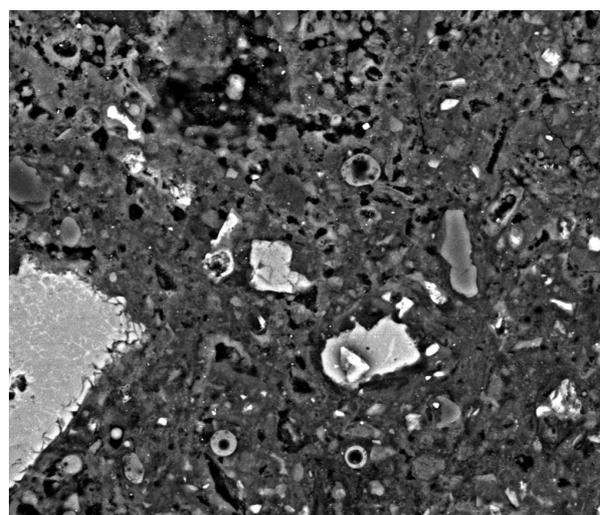
**Figure 20.** BSE image of C1AC after 28 days of hydration (width of field  $\approx 275 \mu\text{m}$ ).
