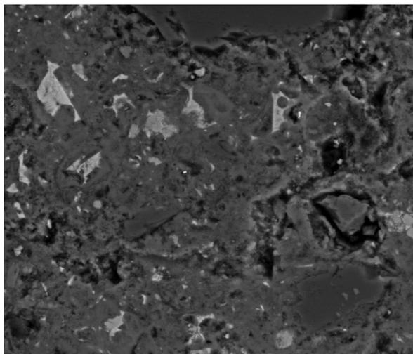
**Figure 18.** BSE image of C1SC after 28 days of hydration (width of field  $\approx 275 \mu\text{m}$ ).
