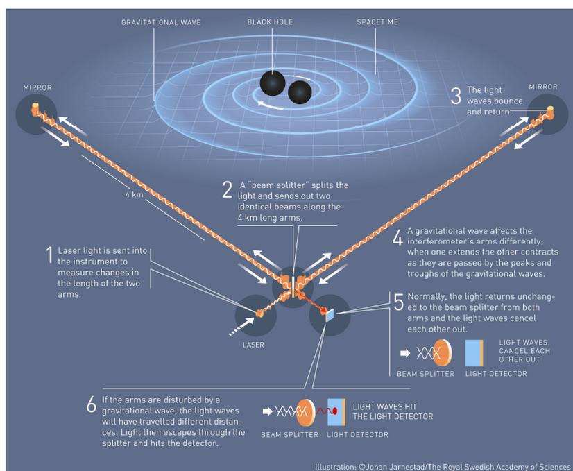
**Figure 1.** The LIGO interferometer is the most sensitive length-measurement device constructed by the humankind.
