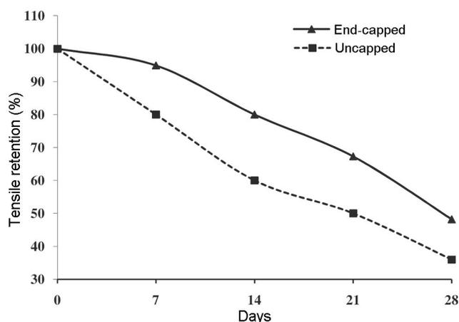
**Figure 13.** Tensile retention (%) of end-capped and uncapped PGCL-copolymer at pH 10.0.
