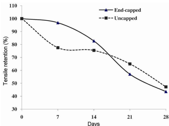
**Figure 12.** Retention (%) of tensile strength at pH 7.4.
