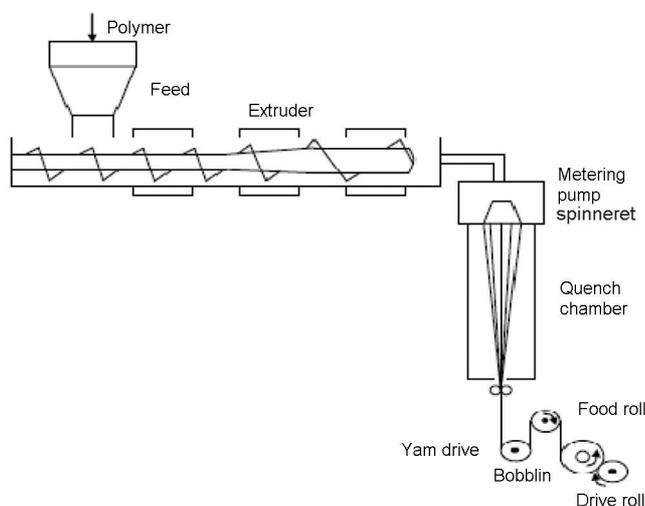
**Figure 2.** Melt spinning line.
