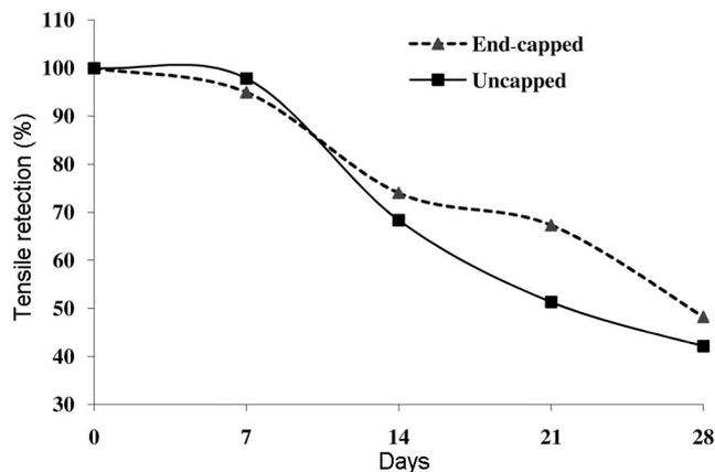
**Figure 10.** Retention (%) of tensile strength at pH 3.2.
