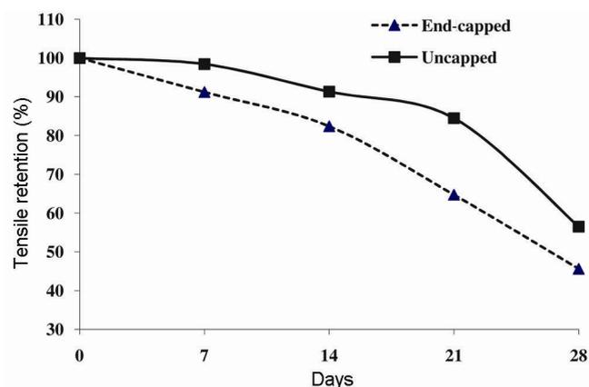
**Figure 11.** Retention (%) of tensile strength at pH 6.4.
