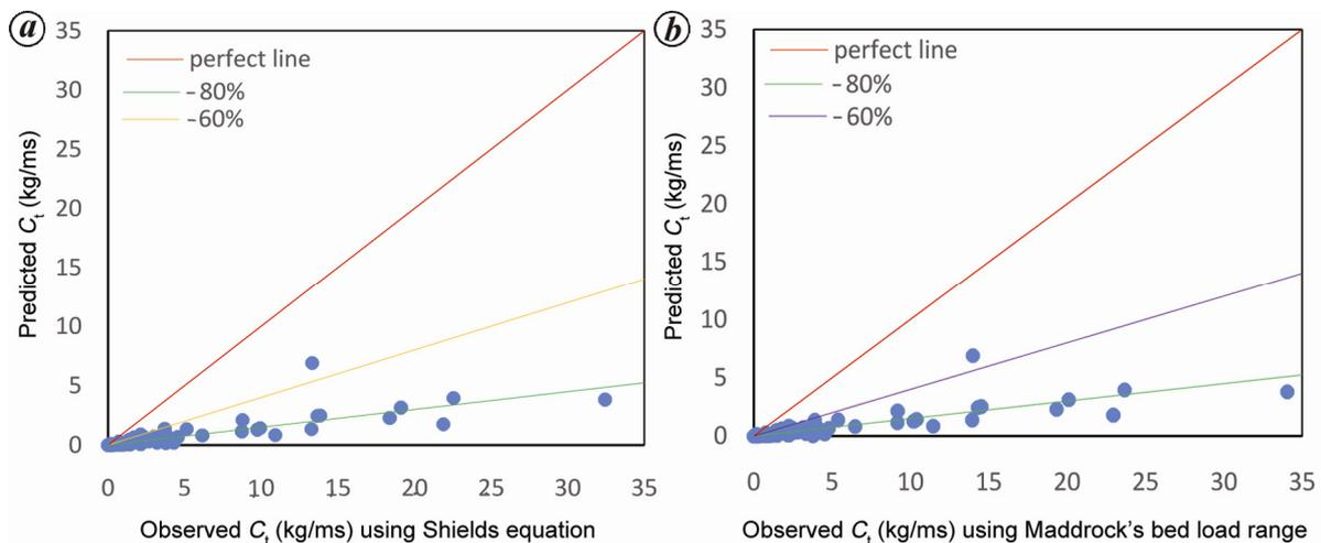
**Figure 3.** Percentage error between observed and predicted total load transport using (a) Shields' equations and (b) Maddock range as bed load for Yang<sup>25</sup> approach.
