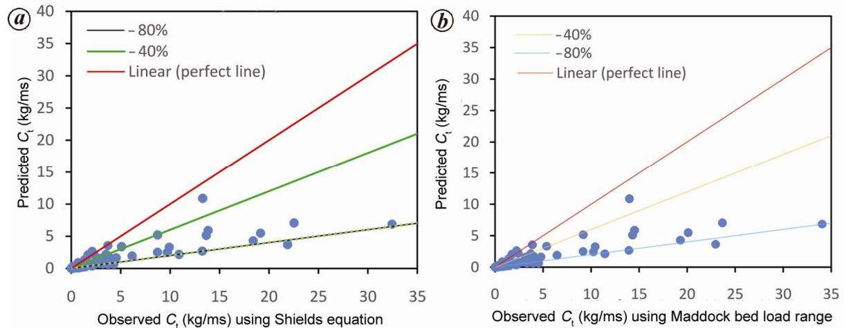
**Figure 2.** Percentage error between observed and predicted total load transport using (a) Shields' equations and (b) Maddock's range as bed load for Yang approach<sup>24</sup>.
