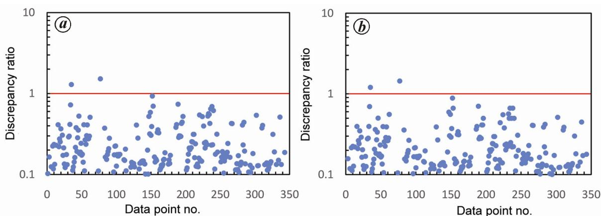
Figure 5. Verification of Yang<sup>25</sup> Unit Stream Power for Shetrunji River data using (a) Shields' bed load formula and (b) Maddock's bed load range.
