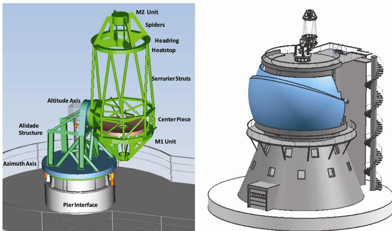
Figure 2. (Left) Overview of the telescope structure. (Right) Telescope and tower with the dome retracted.
