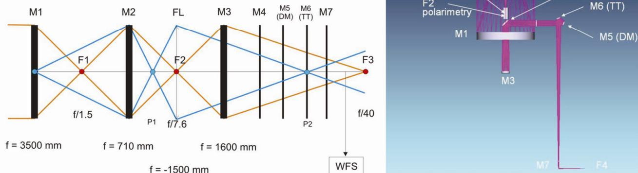
Figure 1. (Left) NLST optical scheme and (right) schematic optical layout.
