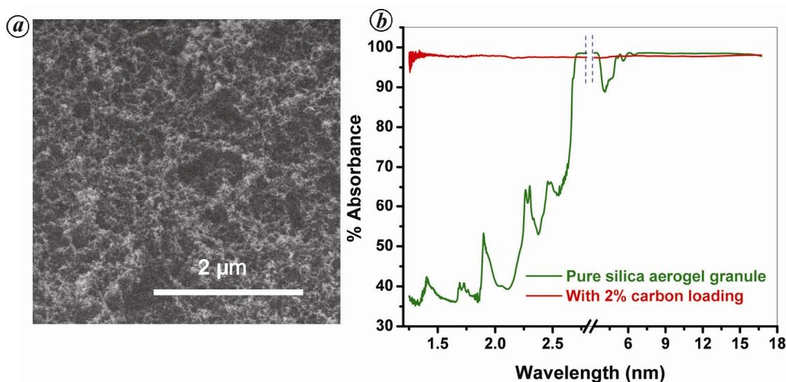
**Figure 5.** *a*, Porosity in silica aerogel granules as seen in SEM image. *b*, Infrared absorption of carbon containing silica aerogel granules.
