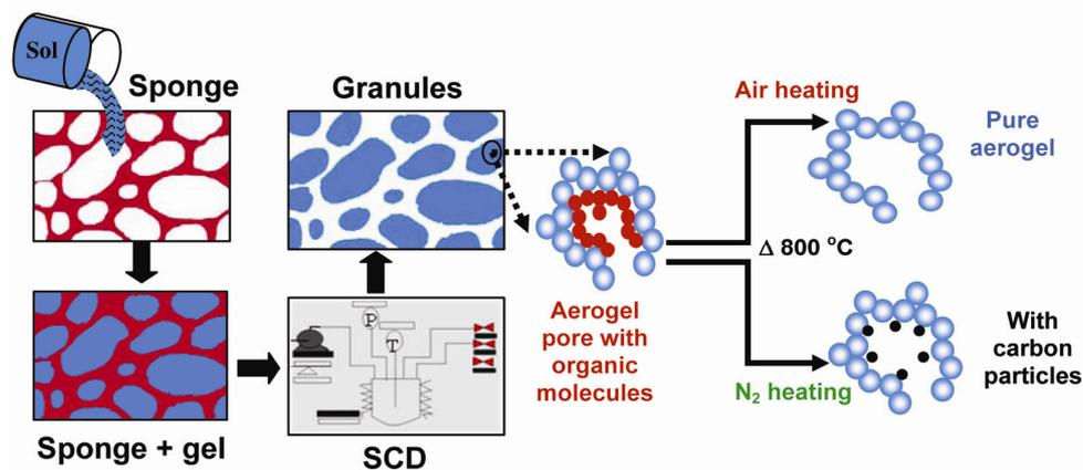
**Figure 4.** Schematic representation of the process of producing pure and carbon-containing silica aerogel granules.
