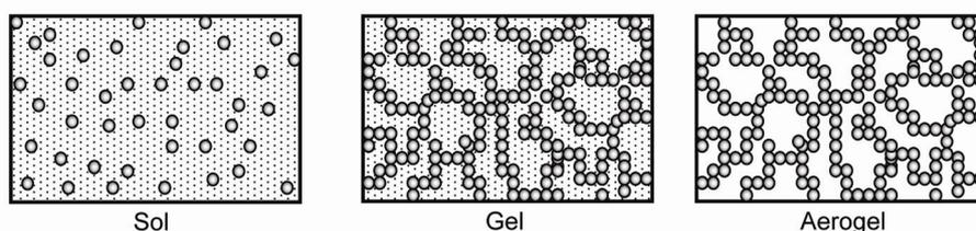
Figure 3. Schematic representation of sol-gel aerogel.
