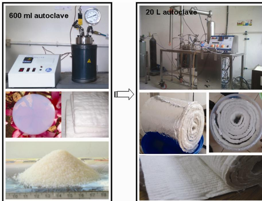
**Figure 6.** Up-scaling of silica aerogel product development from a small 600 ml autoclave to a 20 l autoclave and photographs of the products at the respective scales.
