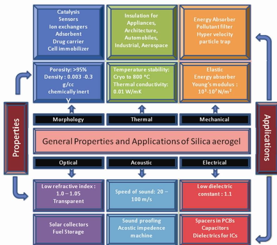
Figure 2. General properties and applications of silica aerogel.
