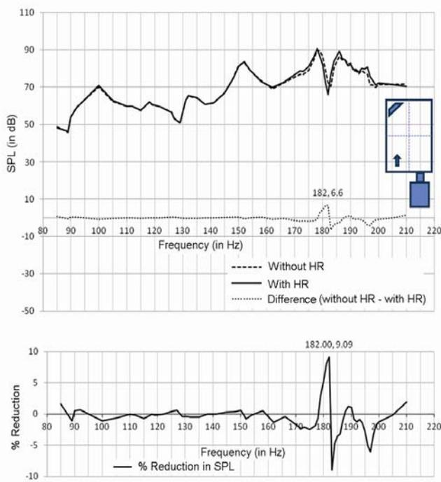
**Figure 3.** (Top) Sound pressure level (SPL) versus excitation frequency. (Bottom) Percentage reduction in SPL. Designed Helmholtz resonator (HR) frequency is 182 Hz. (Inset) Relative position of the speaker, microphone (arrow) and resonator in the enclosure.
