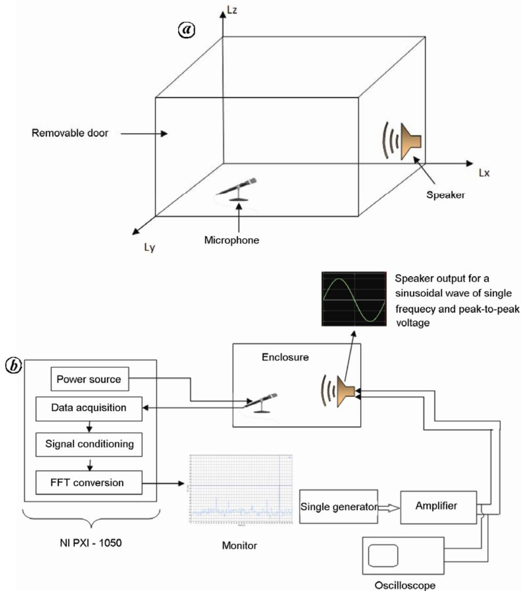
**Figure 1.** Schematic of the experimental set-up: *a*, Enclosure ( $L_x = 1.835$  m,  $L_y = 1.184$  m and  $L_z = 1.1$  m); *b*, Instrumentation employed in the measurements.
