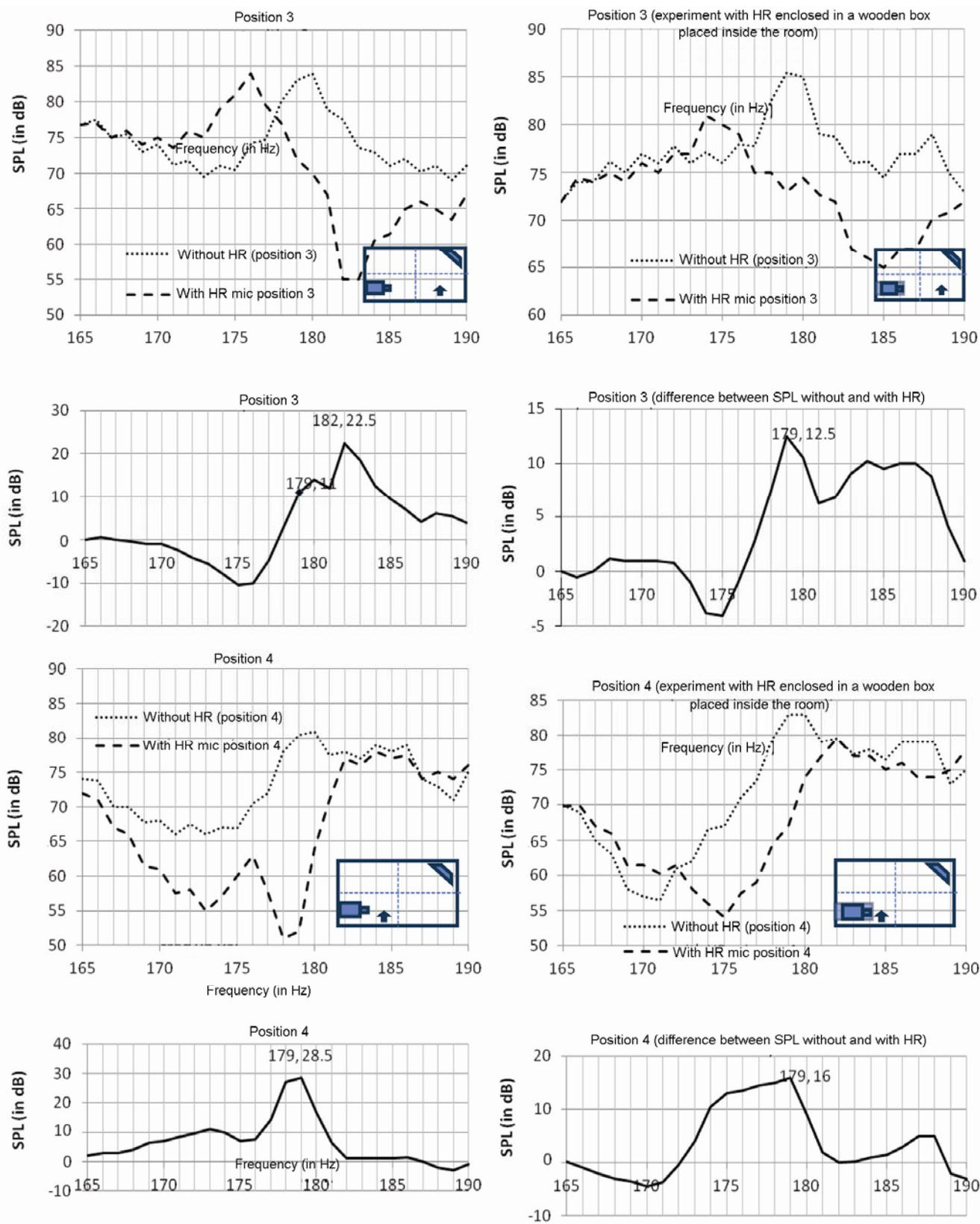
**Figure 11.** SPL versus excitation frequency. The percentage reduction in SPL is also plotted. (Inset) Relative position of the speaker, microphone (arrow) and resonator in the enclosure. The first column from top to bottom are experiments done with only the HR having natural frequency = 178 Hz at various positions of the microphone. The second column are experiments done with HR enclosed in a wooden box at the same location. Readings are for various positions of the microphone.
