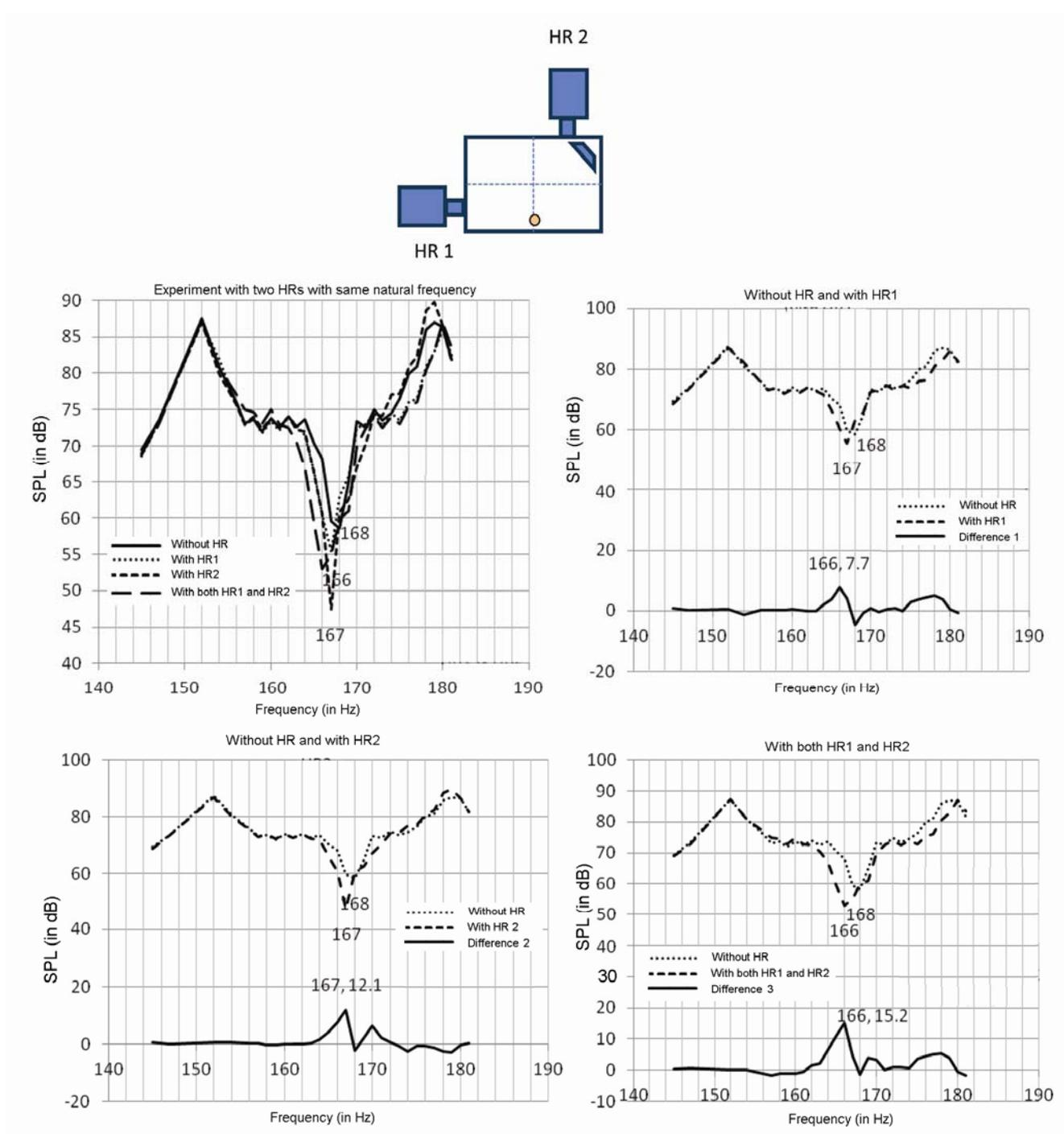
**Figure 10.** SPL versus excitation frequency for HR1 and HR2 and their combination thereof. The percentage reduction in SPL is also plotted. The designed HR frequency is 166 Hz. (Top) Schematic diagram shows the relative position of the speaker, microphone (dot) and resonator in the enclosure.
