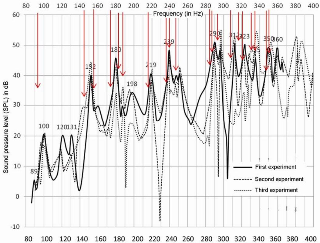
**Figure 2.** Frequency versus amplitude plot for the enclosure. Vertical arrows show the position of theoretically calculated eigenfrequencies of the enclosure. Peaks denote the experimentally obtained resonance at the respective modes. Three experiments were carried out for the range of frequencies with the source fixed at a particular point while the microphone was placed at three different locations.
