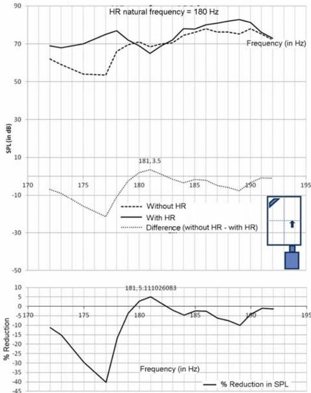
**Figure 5.** (Top) SPL versus excitation frequency. (Bottom) Percentage reduction in SPL. The designed HR frequency is 180 Hz. (Inset) Relative position of the speaker, microphone (arrow) and resonator in the enclosure.
