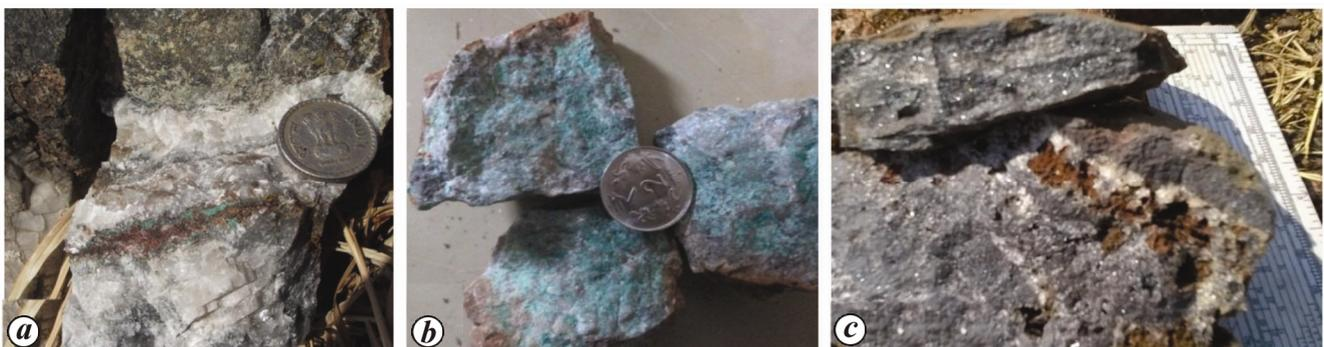
Figure 2. Hand specimens of mineralized zone. a, Malachite stain within calcite vein. b, Malachite-rich quartz vein. c, Alternate specularite and calcite layers containing base metal sulphides.
