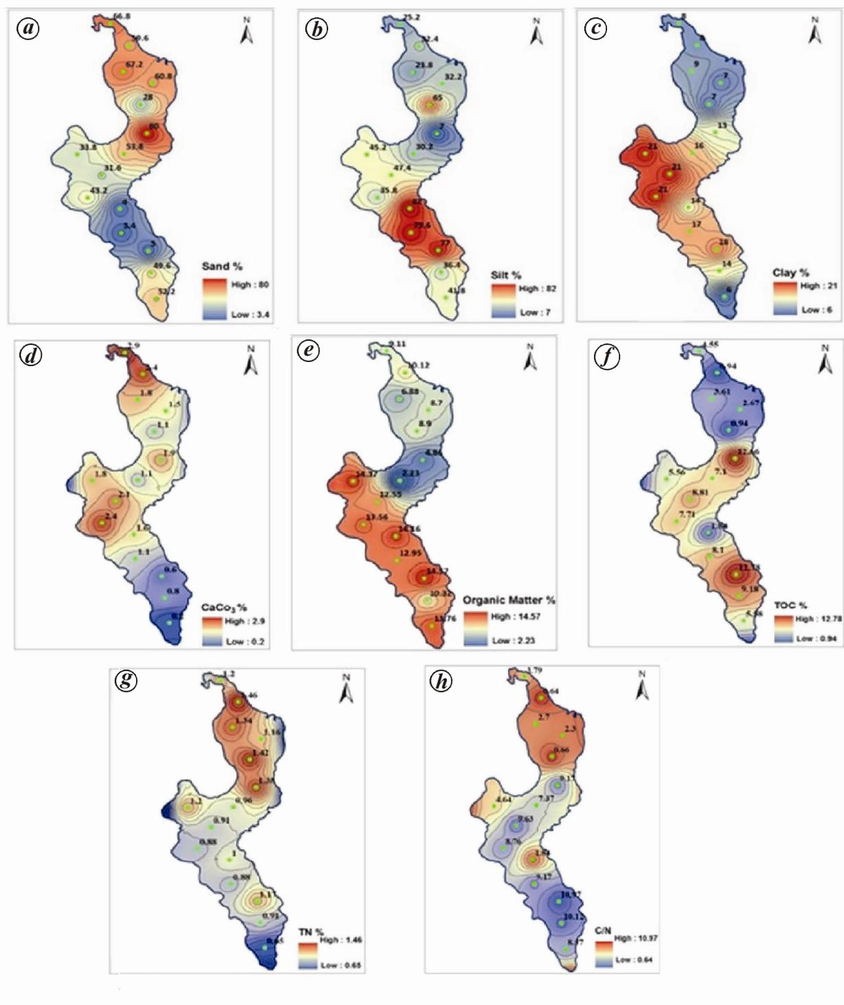
**Figure 5 a–h.** Spatial distribution map of sand, silt, clay,  $\text{CaCO}_3$ , OM, TN and C/N ratio of Kukkal lake.
