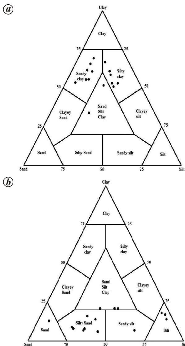
Figure 3. Ternary plot showing relative percentage of sand, silt and clay particles of (a) Berijam lake and (b) Kukkal Lake floor sediments.
