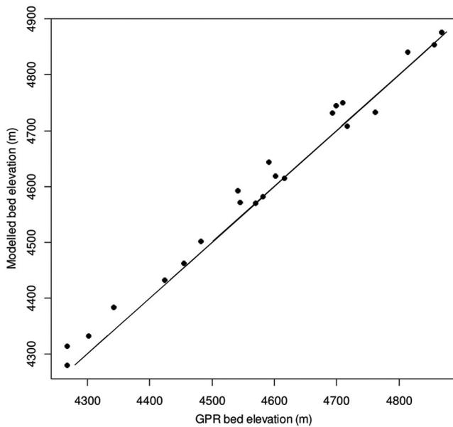
**Figure 4.** Scatterplot showing good correlation between GPR and modelled bed elevation values of Chhota Shigri ( $r = 0.99$ ).
