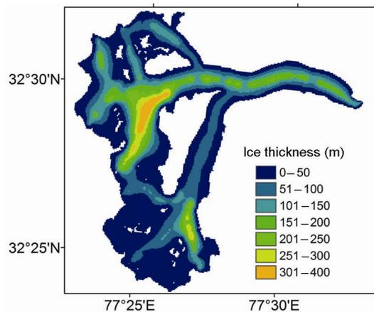
**Figure 6.** Maximum ice thickness of  $\sim 350 \text{ m}$  observed for Samudra Tapu.
