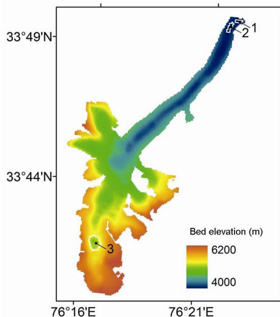
**Figure 7.** Three potential lake sites identified for Drang Drung with mean depth varying between 40 and 75 m.
