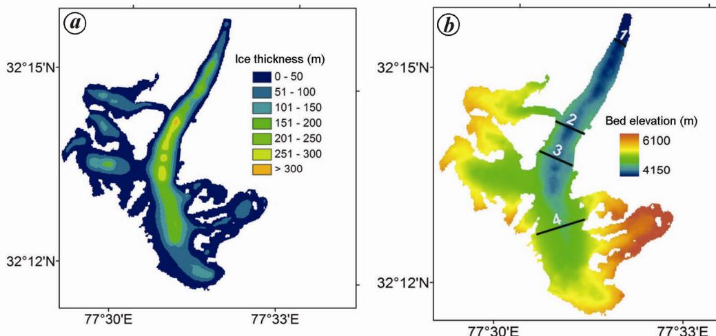
**Figure 2.** *a*, Maximum ice thickness of ~300 m observed for Chhota Shigri. *b*, The four profiles shown are used to compare the modelled bed profiles with the GPR bed profiles.
