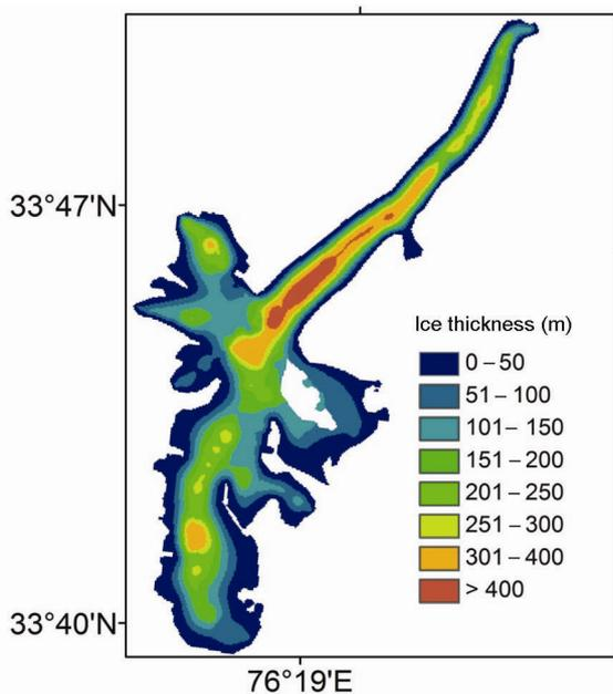
**Figure 5.** Ice thickness of Drang Drung varying from  $\sim 100 \text{ m}$  at the snout to  $>400 \text{ m}$  in the mid-ablation region.
