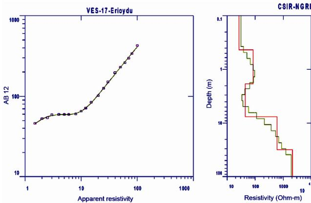
**Figure 2.** a, Logarithm plot between electrode spacing and apparent resistivity (circle indicates field data and continuous line indicates field curve). b, VES interpreted smooth (green line) and layered curves (red line) through the computer 1X1-D Interpex software.
