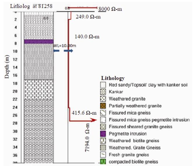
**Figure 5.** Bore hole lithologs (81258) compared with geoelectrical layer parameters and groundwater level at VES\_9 (Mullipadi village in Tamil Nadu)
