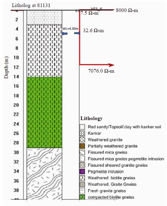
**Figure 4.** Comparison of geoelectrical parameters (at VES\_6) with the existing borehole lithologs (81131) along with water level at Thottumattu village in the study area.
