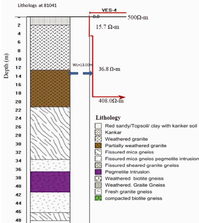
**Figure 3.** Comparison of geoelectrical parameters (at VES\_4) with the existing borehole lithologs (81041) at Sivalsragu village.
