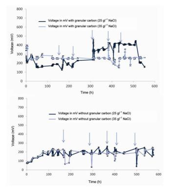
Figure 4. Voltage readings (arrows show spiking with acetate dose).
