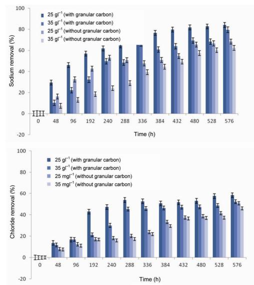
Figure 6. Removal percentage of sodium and chloride.
