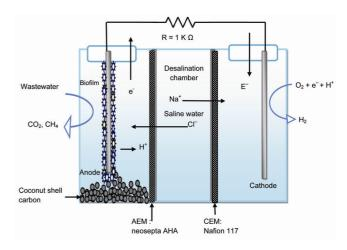
Figure 1. Schematic representation of MDC.
