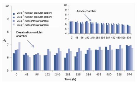
Figure 2. pH values recorded in the desalination chamber and the anode chamber (inset).
