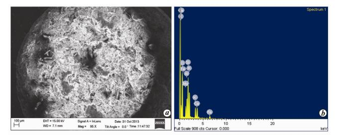
Figure 7. Biofilm on electrode; SEM and energy dispersive X-ray analysis (EDX).
