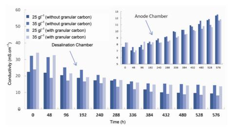
Figure 3. Conductivity readings recorded in the desalination chamber and the anode chamber (inset).
