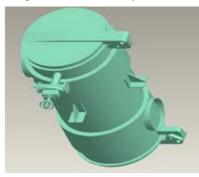
In this the mixed juice is heated in a vertical tubular container up to 60-65 ° C
